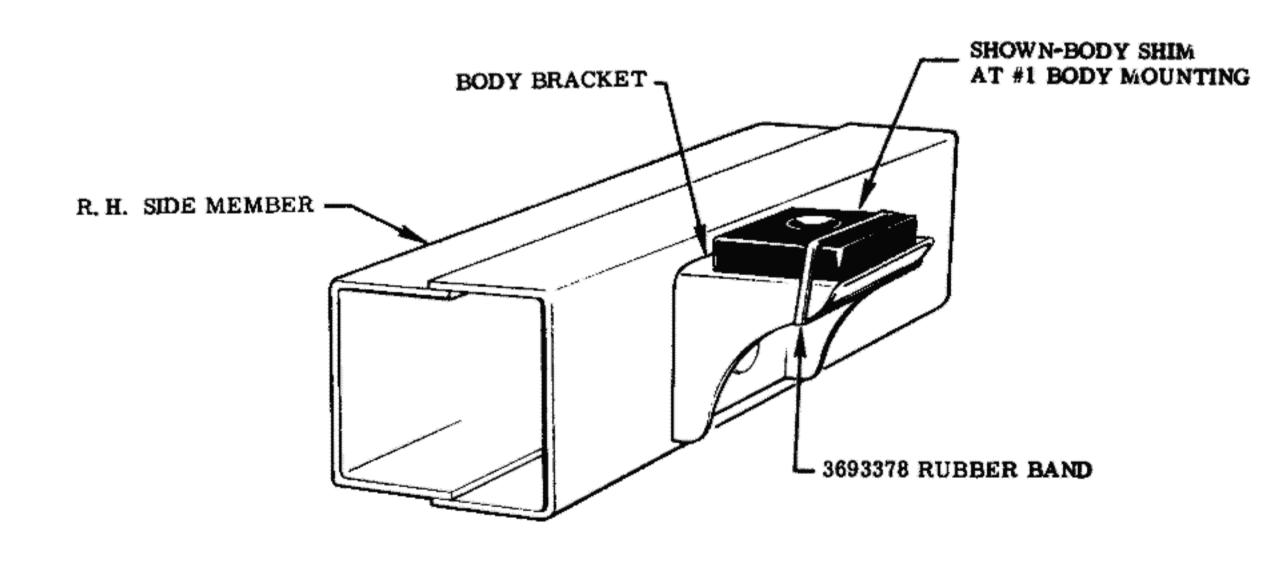
USED TO ATTACH BODY SHIM TO BODY BRACKETS AT #1, #2 OUTER, #3 INNER & OUTER, #3A, #4, #5 & #5A.
