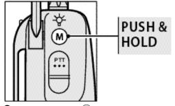
**1** Push and hold the **M** button to allow all signals to enter.
