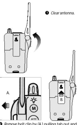
Remove belt clip by (A.) pulling tab out and (B.) Sliding belt clip up and off unit.
