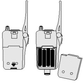
Pull lock tab down and lift door up (towards you) to remove battery cover. Insert four "AAA" batteries. Position batteries according to polarity markings.
