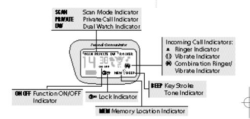
If you push and hold the button, the MicroTalk will cycle through the different functions.
