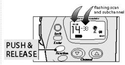
1 Push and release button and subchannel and scan icon will flash.
