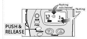
6 Push and release button which sets main channel in memory and moves to subchannel selection. The subchannel begins flashing. The hicon will remain flashing.
