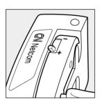
If you do not hear dialtone, adjust the height of the Lifter Arm by moving the Height Control towards "+" to raise the arm. Moving the Height Control towards " -" lowers the arm.
