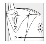
press the Handset Lifter Button on your Beltpack or Headset. When using a non- Beltpack wireless headset, hold the Handset Lifter Button down for 2-3 seconds
