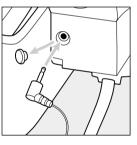
If your telephone's speaker is not under the handset, use the External Sensor. Remove the rubber cover and plug the External Sensor into the External Sensor Port. Peel the tape backing off the External Ring Sensor and attach it over the speaker.
