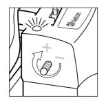
Adjust the Ring Sensor Sensitivity by turning the knob clockwise to increase the sensitivity and counterclockwise to decrease the sensitivity. While the phone is ringing, turn the knob until the Ring Sensor LED lights. Stop turning as soon as the LED lights for optimal performance.
