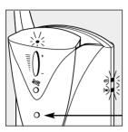
5. Press the Handset Lifter Button\* on your Beltpack or Headset to put the wireless system in Headset Mode and activate the Lifter. The Lifter may take a moment
