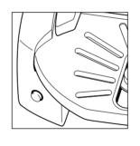
When using the speakerphone feature on your telephone, press the Ring Sensor On/Off Button to disable it. When disabled, the Ring Sensitivity LED rapidly flashes.
