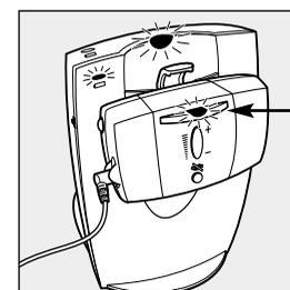
5. Slide the Remote into the Charger on the front of the Base. The Battery Charge light on the front of the Base illuminates. Charge the Battery for a full 3 hours. You may use the handset while the Battery charges.
