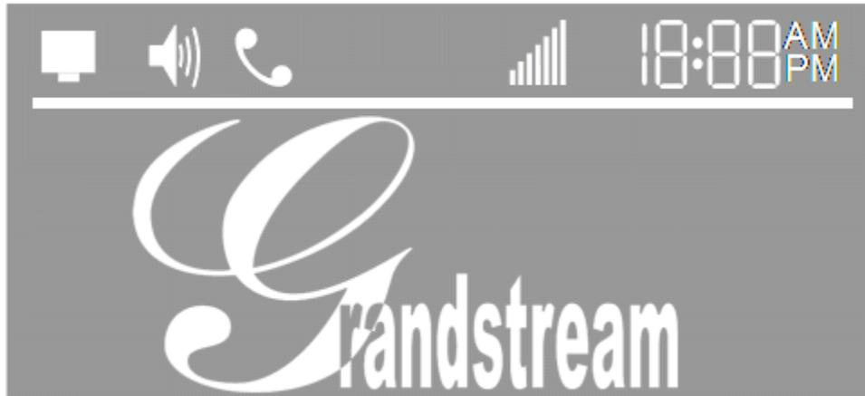
The LCD is equipped with a backlight. When the phone is configured properly and in the normal idle state, the backlight is off. Whenever an event occurs, the backlight turns on automatically and brings the user's attention.
