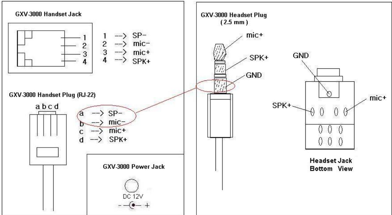
As show in the schema, the left side is pin assignment of a RJ-22 handset plug; while the right side is showing a normal 2.5mm headset plug. If use want to connect the phone to external Speaker or Intercom/Paging system, necessary adaptors are required from local electronic stores.
