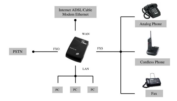
HandyTone-488 has one FXS port and one FXO port. The PHONE port next to the LAN port is a FXS port. The LINE port on the side of the HandyTone-488 is a FXO port. Both the FXS port and the FXO port can have a separate SIP account. This is a key feature of HandyTone-488 as it supports simultaneous call on both FXS port and FXO port. Telephone calls can be originated from or terminated on the PSTN network via FXO port remotely.
