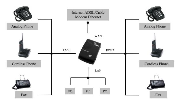
HandyTone-496 has two FXS ports. The PHONE1 port next to the LAN is FXS port 1 and the PHONE2 on the side of the HandyTone-496 is FXS port 2. Each FXS port can have a separate SIP account. This is a key feature of HandyTone-496. Both ports can make calls concurrently.
