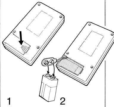
Press down on center of cover. Slide cover out to remove.
