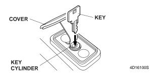
• Turn the key clockwise. The cylinder comes up and unlocks.
