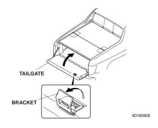
**NOTICE**: Be careful not to damage the tailgate bracket during loading and unloading of cargo.
