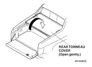
Do not place cargo on the tonneau cover and do not sit on the tonneau cover.
