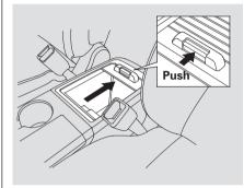
If equipped Push the release knob to open or close the console compartment, slide the lid rearward.
