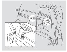
On LX model Your vehicle also has cargo hooks on side panel in the cargo area.
