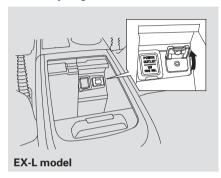
Your vehicle has the auxiliary input jack on the front panel, on the center table, or in the console compartment, depending on models. The system will accept auxiliary input from standard audio accessories.
