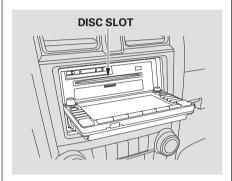
Insert a disc about halfway into the disc slot. The drive will pull the disc in the rest of the way and begin to play it.
