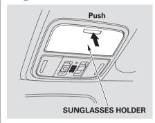
To open the sunglasses holder, push on the raised detent. It will unlatch and swing down. To close it, push it until it latches. Make sure the holder is closed while you are driving.
