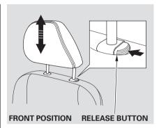
The head restraints adjust for height. You need both hands to adjust a restraint. Do not attempt to adjust it while driving. To raise it, pull upward. To lower the restraint, push the release button sideways, and push the restraint down.
