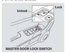
To lock all doors and the tailgate, push the front of the master door lock switch on either front door, pull the lock tab rearward on the driver sdoor, or use the key on the outside lock on the driver s door.
