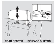
When a passenger is seated in the rear center seating position, make sure the center head restraint is properly adjusted.
