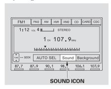
You can adjust the sound on the navigation screen. To adjust the sound, push the AUDIO button, then enter the sound grid by touching the SOUND icon on the display.
