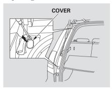
1. Open the tailgate. Place a cloth on the edge of the cover. Remove the covers by carefully prying on the edge with a small flat-tip screwdriver.
