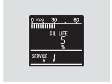
When the remaining engine oil life is 5 to 1 percent, you will see a "SERVICE" message along with the same maintenance item code(s), every time you turn the ignition switch to the ON (II) position.
