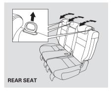
The angle of each rear seat-back can be adjusted separately. To change the seat-back angle of the rear seat-back, pull up on the release lever on the top of the seat-back. Move the seat-back to the desired position, then release the lever. Make sure the seat-back latches in the new position.
