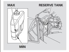
Look at the coolant level in the radiator reserve tank. Make sure it is between the MAX and MIN lines. If it is below the MIN line, see **Adding Engine Coolant** on page 270 for information on adding the proper coolant.
