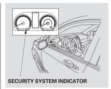
Once the security system is set, opening any door without using the key or the remote transmitter, the hood, or the tailgate will cause the system to alarm.
