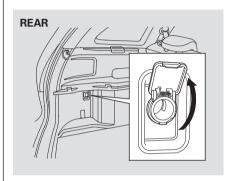
Make sure to put the socket cover back in place to prevent any small foreign objects getting into the socket.
