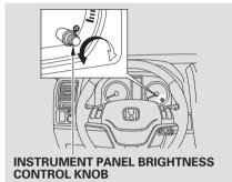
You can change the instrument panel brightness only when the light switch is on.
