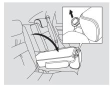
The rear center seat-back has an armrest. To use it, fold it down. To use the cargo area pass-through, pull up the release on top of the center seat-back and fold it down.
