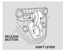
To shift from any position, press firmly on the brake pedal and press the release button on the side of the shift lever. You cannot shift out of Park when the ignition switch is in the LOCK (0) or ACCESSORY (I) position.
