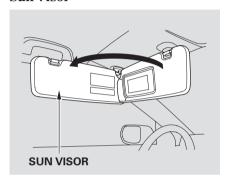
To use the sun visor, pull it down. When using the sun visor for the side window, remove the support rod from the clip, and swing it out.
