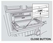
To return the screen to the upright position, press the CLOSE button on the edge of the screen panel. Do not use the folded screen as a tray. If you put a cup, for example, on the screen, the liquid inside the cup may spill on the screen when you go over a bump.
