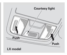
Turn on the spotlight by pushing the lens. Push the lens again to turn it off. You can use the spotlights at all times.
