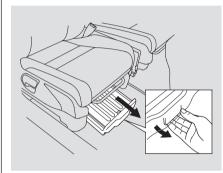
If equipped Your vehicle has a seat under tray located under the front passenger seat. Use the tray by pulling on the front center edge of the tray.
