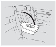
On vehicles with rear seat armrest The rear seat also has a beverage holder in the center armrest. To use it, pivot the armrest down.
