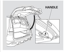
Keep the tailgate closed at all times while driving to avoid damaging the tailgate and to prevent exhaust gas from getting into the interior. See **Carbon Monoxide Hazard** on page 54.
