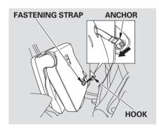
5. Pull down on the anchor to engage the upper part of the anchor securely on the hook, and make sure the seat is secure. Make sure that the folded up right rear seat does not interfere with the front passenger's seat-back. This will cause the front passenger's weight sensors and the front passenger's seat belt reminder indicator to work improperly (see page 32). Also check the passenger airbag off indicator to assure proper operation of the passenger's advanced front airbag.
