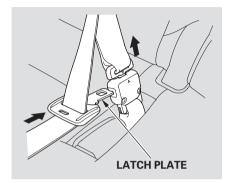
When you are folding the rear center seat-back, use the latch plate to release the center seat belt from the detachable anchor (see page 104). Allow the seat belt to retract into the holder on the ceiling and store the buckles in it.
