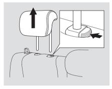
5. Remove the head restraint (see page 97). Make sure the removed head restraint is secured in the cargo area.
