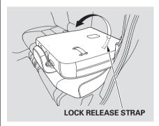
3. Unlock the seat from the floor by pulling the lock release strap under the seat cushion's back edge, then lift the rear of the seat. You cannot fold up the rear seat if it is not latched securely in the rearmost position.
