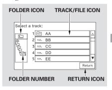
You can also select a track/file directly from a track list on the audio display. Press the AUDIO button to show the audio display, then touch the Track List icon. The track list menu appears on the display.
