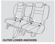
To install a LATCH-compatible child seat in either of the rear outer seats:
