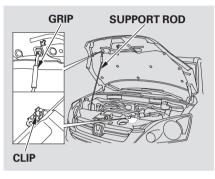
3. Holding the grip, pull the support rod out of its clip. Insert the end into the designated hole pointed by an arrow in the hood.
