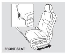
To adjust the front or rear seat forward and backward, pull up on the bar under the seat cushion's front edge. Move the seat to the desired position, and release the lever. Try to move the seat to make sure it is locked in position.
