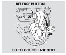
6. Remove the key from the shift lock release slot, then reinstall the cover. Make sure the notch on the cover is on the right side. Press the brake pedal, and restart the engine.
