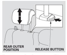
To remove a head restraint, pull it up as far as it will go. Push the release button, then pull the restraint out of the seat-back.
