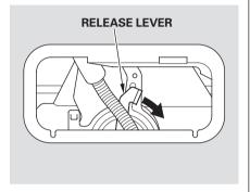
Push the release lever to the lower right as shown.
