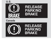
If you start driving without releasing the parking brake, the multi-information display interrupts the current display and shows "RELEASE PARKING BRAKE." This message continues, and a chime sounds, until you release the parking brake, or the vehicle speed slows down to less than 0.5 mph (0.8 km/h).
