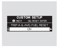
Press the SEL/RESET button. The display changes as shown above. The lower segment changes between "ON" and "OFF" each time you press the INFO button. Enter your selection by pressing the SEL/RESET button.
