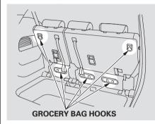
The grocery bag hooks on the back of the third row seats are designed to hold plastic grocery bags containing lightweight items. Heavy objects may damage the hooks. **Before Driving**
