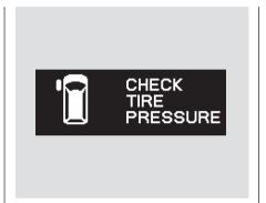
The TPMS monitors the air pressure of all four tires whenever the ignition switch is in the ON (II) position. It will immediately sense if a tire starts to lose its pressure, and give you warning with the low tire pressure indicator in the instrument panel and a "CHECK TIRE PRESSURE" message on the multi-information display. If the indicator and the warning message do not come on again after you inflate the tire to its correct air pressure (see page 384),
