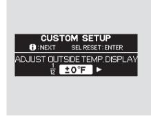
Press the SEL/RESET button. The display changes as shown above. The highlighted number is the current adjustment above or below the outside temperature. Press the INFO button repeatedly until the appropriate number appears, then press the SEL/RESET button to enter your selection.
