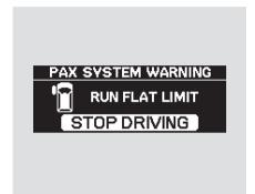
If you see the above message on the multi-information display, you have reached the limit of run flat driving, and you should stop driving immediately. Be aware that if you continue to drive, the noise and vibration level from the tire will increase significantly, and the tire may no longer be repairable.
