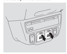
There are three accessory power sockets in your vehicle. Two accessory power sockets are above the center pocket for the front seat passengers, and another is on the cargo area sidewall on the driver's side.
