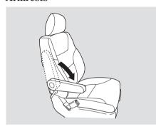
An armrest is located on each of the front seats and on each side of the second row seats. Pivot it down to use it. When you remove the bucket seats in the second row, pivot the armrests up out of the way.
