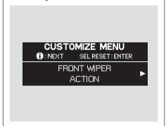
With "WIPER SETUP" shown on the multi-information display, press the SEL/RESET button on the steering wheel. The display changes to "FRONT WIPER ACTION" as shown above.
