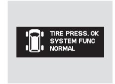
To display the tire pressure monitor, press the INFO button until it appears on the multi-information display.
