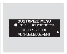
While the multi-information display shows "DOOR-WINDOW SETUP," press the SEL/RESET button on the steering wheel. Then press the INFO button repeatedly until you see "KEYLESS LOCK ACKNOWLEDGEMENT" as shown above.
