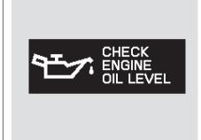
If the engine oil is very low or has lost pressure, you will see "CHECK ENGINE OIL LEVEL" on the multiinformation display. You will also see the low oil pressure indicator in the instrument panel flashing or staying on. If you see this message, you should take immediate action since serious engine damage is possible. Follow the procedure on page 409.
