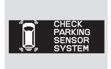
message. Check the sensors first. If the message stays on or the beeper does not stop, have the system checked by your dealer.
