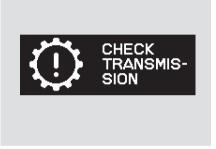
If there is a problem with the automatic transmission, you will see "CHECK TRANSMISSION" on the multi-information display. Avoid rapid acceleration, and have the transmission checked by a dealer as soon as possible.
