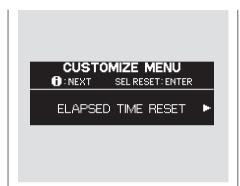
While the multi-information display shows "METER SETUP" of the "CUSTOMIZE GROUP," press the SEL/RESET button on the steering wheel. The display changes to "CUSTOMIZE MENU." Press the INFO button repeatedly until you see "ELAPSED TIME RESET" in the lower segment as shown above.
