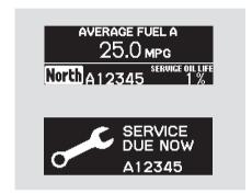
When the remaining engine oil life is less than 5 percent, you will see the above display. The display then changes to "SERVICE DUE NOW." Have the indicated maintenance done as soon as possible.
