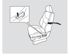
To change the seat-back angle of the front seat, pull up the lever on the outside of the seat bottom.
