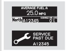
When the remaining engine oil life is less than 0 percent and you have not done the required maintenance, you will see the above display for several seconds. In this display, "0" will be blinking.
