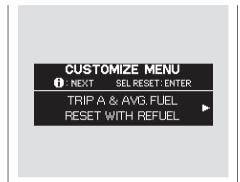
While the multi-information display shows "METER SETUP" of the "CUSTOMIZE GROUP," press the SEL/RESET button on the steering wheel. The display changes to "CUSTOMIZE MENU." Press the INFO button repeatedly until you see "TRIP A & AVG. FUEL RESET WITH FUEL" in the lower segment as shown above.
