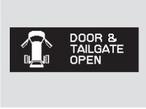
The door and tailgate open monitor appears on the multi-information display to indicate when a specific door or the tailgate is not tightly closed.
