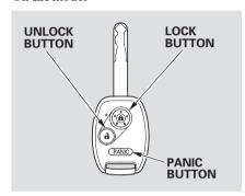
LOCK — Press this button once to lock all doors and the tailgate. Some exterior lights will flash once. When you push LOCK twice within 5 seconds, you will hear a beep to verify that the security system has set. You cannot lock the doors and the tailgate if any door or the tailgate is not fully closed or the key is in the ignition switch.
