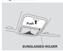
To open the sunglasses holder, push on the raised detent. It will unlatch and swing down. To close it, push it until it latches. Make sure the holder is closed while you are driving.
