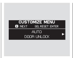
While the multi-information display shows "DOOR-WINDOW SETUP," press the SEL/RESET button on the steering wheel. Then press the INFO button once. The display changes to "AUTO DOOR UNLOCK" as shown above.
