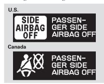
If the passenger's side airbag has automatically shut off, you will see "PASSENGER SIDE AIRBAG OFF" on the multi-information display. See page 35 for more information.
