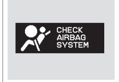
If there is a problem with your front airbags, side airbags, passenger's side airbag automatic cutoff system, automatic seat belt tensioners, side curtain airbags, driver's seat position sensor, or the front passenger's weight sensors, you will see "CHECK AIRBAG SYSTEM" on the multi-information display. Take your vehicle to a dealer as soon as possible (see page 34).
