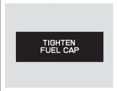
Your vehicle's on board diagnostic system will detect a loose or missing fuel fill cap as an evaporative system leak. The first time a leak is detected a "TIGHTEN FUEL CAP" message appears on the multi-information display. Turn the engine off, and confirm the fuel fill cap is installed. If it is, loosen it, then retighten it until it clicks at least once. The message should go off after several days of normal driving once you tighten or
