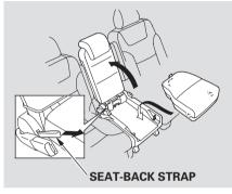
Hook the front of the seat to the floor, then push down the back until it locks. Make sure both the front and back of the seat are securely latched. Pull up the seat-back, and adjust the seat-back angle to the desired position while pulling the seat-back strap on the outside of the seat bottom.
