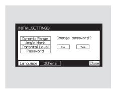
If you forget the password, select "Password," and press the ▲ button 10 times.
