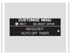
While the multi-information display shows "LIGHTING SETUP," press the SEL/RESET button on the steering wheel. Then press the INFO button to display "HEADLIGHT AUTO OFF TIMER" as shown above.
