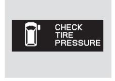
When any of the tires have low pressure, the low tire pressure indicator on the instrument panel comes on, and the multi-information display also interrupts the current display and shows a "CHECK TIRE PRESSURE" message. You can see one or more of the low pressure tire positions highlighted in the display along with this message.
