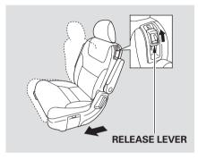
To get into or out of the third row seat, pull up the release lever on the shoulder of each second row bucket seat. The seat-back will tilt forward and the whole seat will slide forward.
