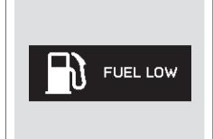
If the level of the fuel in the tank gets low, you will see "FUEL LOW" on the multi-information display, and you must refuel soon. The low fuel indicator on the instrument panel will also come on.
