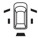
The appropriate light comes on in this monitor if the tailgate or any door is not closed tightly.
