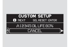
5. If you want to cancel resetting, press the INFO button on the steering wheel. The display changes as shown. Press the SEL/RESET button. This cancels the resetting procedure, and the screen returns to the normal display mode.
