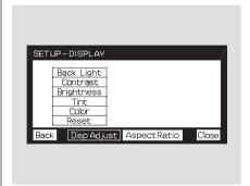
If you want to set the display to the default setting, select "Reset" by pressing the ▼ or ▲ button, and, then pressing the ENT button.
