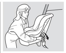
1. With the child seat in the desired seating position, route the belt through the child seat according to the seat maker's instructions, then insert the latch plate into the buckle.
