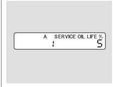
When the remaining engine oil life is 5 to 1 percent, you will see a "SERVICE OIL LIFE" message along with the same maintenance item code(s), every time you turn the ignition switch to the ON (II) position.
