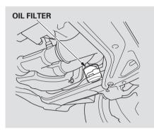
3. Remove the oil filter, and let the remaining oil drain. A special wrench (available from your dealer) is required.
