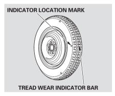
Replace the tire when you can see the tread wear indicator bars. The replacement should be the same size and design tire, mounted on the same wheel. The spare tire is not designed to be mounted on a regular wheel, and the spare wheel is not designed for mounting a regular tire. If you have a flat tire while driving, stop in a safe place to change it. Drive slowly along the shoulder until you get to an exit or an area to stop that is far away from the traffic lanes.
