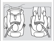
Your vehicle also has side airbags to help protect the upper torso of the driver or a front seat passenger during a moderate to severe side impact (see page 31 for more information on how your side airbags work).
