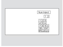
Select and enter the second digit number the same way. The cursor will automatically move to the "ENT" icon when you press the ENT button. Press the ENT button to enter the number command. To go back to the DVD screen, press the RETURN button.
