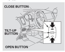
The moonroof has two positions: it can be tilted up in the back for ventilation, or it can be slid back into the roof. Use the switch under the left dashboard vent to operate the moonroof. The ignition switch must be in the ON (II) position.
