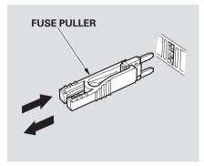
4. Check the smaller fuses in the under-hood fuse box and all the fuses in the interior fuse boxes by pulling out each fuse with the fuse puller.
