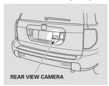
Whenever you shift to R (reverse) with the ignition switch in the ON (II) position, the rear view is shown on the navigation or Compass system screen.
