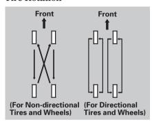
To help increase tire life and distribute wear more evenly, rotate the tires according to the maintenance messages displayed on the information display. Move the tires to the positions shown in the illustration each time they are rotated. If you purchase directional tires, rotate only front-to-back.
