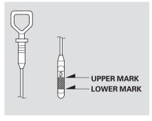
4. Remove the dipstick again, and check the level. It should be between the upper and lower marks.
