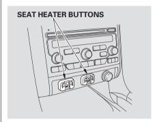
Push the top of the switch, HI, to rapidly heat up the seat. After the seat reaches a comfortable temperature, select LO by pushing the bottom of the switch. This will keep the seat warm.
