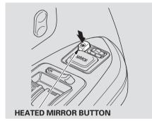
The outside mirrors are heated to remove fog and frost. With the ignition switch in the ON (II) position, turn on the heaters by pressing the button. The indicator in the button comes on as a reminder. Press the button again to turn the heaters off.
