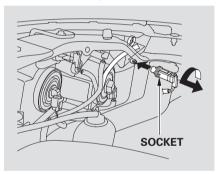
1. Remove the socket from the headlight assembly by turning it one-quarter turn counterclockwise.
