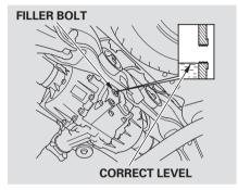
Check the fluid level with the differential at normal operating temperature and the vehicle sitting on level ground. Remove the differential fluid filler bolt and washer, and carefully feel inside the bolt hole with your finger. The fluid level should be up to the edge of the bolt hole. If it is not, slowly add VTM-4 Differential Fluid until it starts to run out of the hole.
