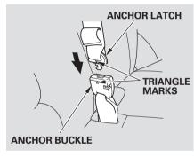
Insert the hook at the end of the anchor latch into the anchor buckle by lining up the triangle marks on the anchor latch and buckle. Make
