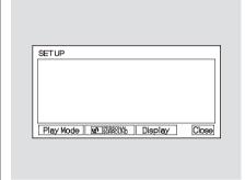
When you press the SETUP button while a DVD is playing, the DVD's setup menu is displayed at the bottom of the screen. You can then change various settings of play mode, personal surround, and display. To go back to play without changing any setting, press the RETURN or SETUP button, or select "Close" by pressing the ▶ or ◀ button, then press the ENT button.
