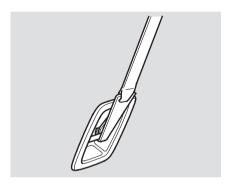
2. Attach the tether strap hook to the anchor, making sure the tether strap is not twisted.
