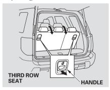
Pull on the handle on the back of the seat-back, move the seat-back to the desired position, and release the handle. Let the seat-back latch in the new position.
