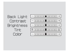
Select the quality you want to adjust by pressing the ▼ or ▲ button, and then pressing the ENT button. The adjustment bar is displayed next to the selected item. Adjust the setting by pressing the ▶ or ◀ button. When you are finished with your adjustment, press the ENT button.
