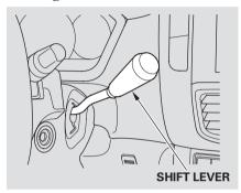
To shift from Park to any position, press firmly on the brake pedal, and pull the shift lever toward you. You cannot shift out of Park when the ignition switch is in the LOCK (0) or ACCESSORY (I) position.
