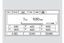
On vehicles with navigation system In addition to the knobs, buttons, and bars on the radio control panel, you can operate some of the radio controls on the navigation system screen. While you are listening to the radio, you can change to another band by pressing the AUDIO button next to the navigation system screen, and then touching the desired band icon (FM1, FM2, or AM).
