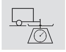
Tongue Load: The weight that the tongue of a fully loaded trailer puts on the hitch should be 5 to 10 percent of the total trailer weight for boat trailers, and 8 to 15 percent of total trailer weight for all other trailers. (See page 215 for limits for your towing situation). Too much tongue load reduces front-tire traction and steering control. Too little tongue load can make the trailer unstable and cause it to sway.
