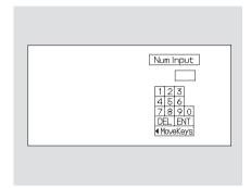
A numerical command can be issued to a DVD by inputting a two digit number, and a button number can be selected on the screen.
