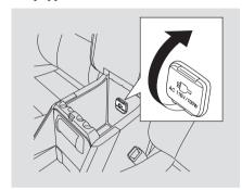
There is a 115 volt AC power outlet in the console compartment. To use the AC power outlet, open the console compartment lid and open the outlet cover. Insert the plug into the receptacle slightly, turn it 90° clockwise, then push in the plug all the way.
