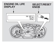
To see the current engine oil life, turn the ignition switch to the ON (II) position, and push and release the Select/Reset knob repeatedly until the engine oil life display appears (see page 70).
