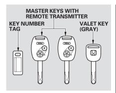
The master key fits all the locks on your vehicle. The valet key works only in the ignition and the door locks. You can keep the glove box locked when you leave your vehicle and the valet key at a parking facility.
