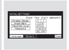
■ button, and enter it by pressing the ENT button. Repeat this until all four numbers are entered. When you enter the fourth number, the cursor automatically moves to "ENT" on the display. Press the ENT button on the control panel.
