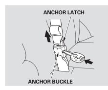
To unlatch the detachable seat belt anchor before folding down the seat-back, insert your ignition key into the slot on the side of the anchor buckle and allow the seat belt to retract. For the center seating positions, place the latch plate and anchor latch into their holding slots in the ceiling. For the third row outer seating positions, re-fasten the belt with the clip.
