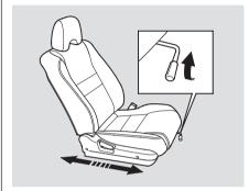
To adjust the seat forward and backward, pull up on the lever under the front seat cushion. Then try to move the seat to make sure it is locked into position.
