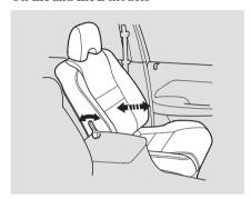
To change the lumbar support, move the lever on the right side of the seat-back forward or backward. Keep moving the lever forward or backward until you find a suitable position.
