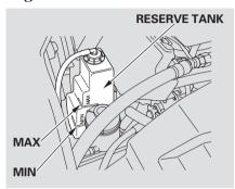
Look at the coolant level in the radiator reserve tank. Make sure it is between the MAX and MIN lines. If it is below the MIN line, see **Adding Engine Coolant** on page 242 for information on adding the proper coolant.
