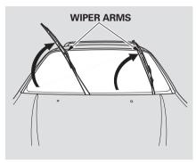
1. Raise each wiper arm off the windshield, lifting the driver's side first, then the passenger's side.
