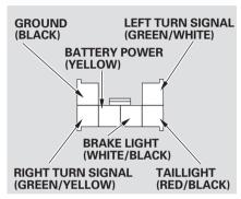
Trailer lights and equipment must comply with federal, state, province, and local regulations. Check trailer light requirements for the areas where you plan to tow, and use only equipment designed for your vehicle. Your vehicle is equipped with a connector to install a trailer lighting connector that mates with your vehicle.
