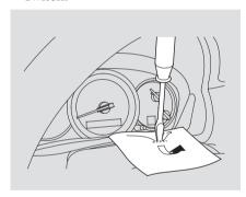
3. Put a cloth on the edge of the shift lock release slot cover. Using a small flat-tipped screwdriver or a metal fingernail file, carefully pry on the edge of the cover to remove it.
