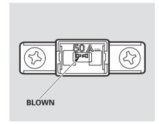
3. Check each of the large fuses in the primary under-hood fuse box by looking through the top at the wire inside. Remove the screws with a Phillips-head screwdriver.
