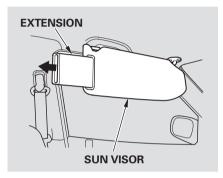
When using the sun visor for the side window, remove the support rod from the clip and swing it out. Slide the extension out to get more coverage on the side window.
