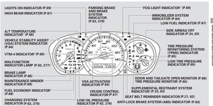
The U.S. instrument panel is shown. Differences for the Canadian models are noted in the text. \* : If equipped.
