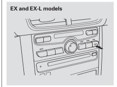
The rear window defogger will clear fog, frost, and thin ice from the window. Push the defogger button to turn it on and off. The indicator above the button comes on to show the defogger is on. If you do not turn it off, the defogger will shut itself off after about 15 minutes. It also shuts off when you turn off the ignition switch. You have to turn the defogger on again when you restart the vehicle.
