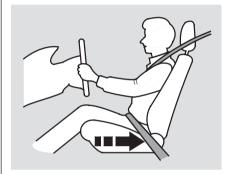
Adjust the driver's seat as far to the rear as possible while allowing you to maintain full control of the vehicle. Have a front passenger adjust their seat as far to the rear as possible.
