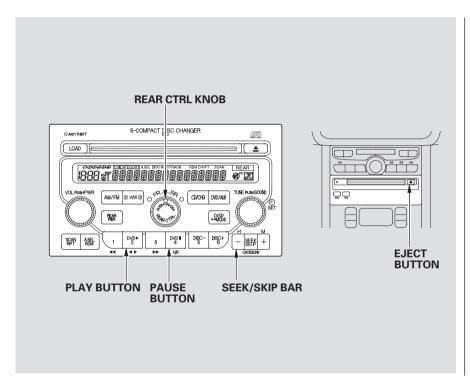
Turn the Rear CTRL knob clockwise. The amber Rear LED comes on to show that the control panel is now enabled.
