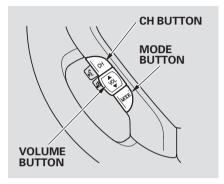
If you are listening to the radio, use the CH button to go to the next preset station. You will see the number of the preset button in the display. To change bands, press the AM/FM button.
