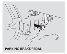
To apply the parking brake, push the pedal down with your foot. To release it, push on the pedal again. The parking brake indicator on the instrument panel should go out when the parking brake is fully released (see page 63).
