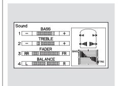
**Treble/Bass** — To adjust the treble and bass, touch + or — on each side of the treble or bass adjustment bar. The adjustment bar shows you the current setting.
