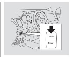
This switch is under the left vent. Press it to turn the vehicle stability assist system on and off.
