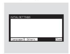
When you press the SETUP button on the rear control panel when a DVD is not playing, the "INITIAL SETTINGS" menu is displayed.
