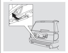
To open the tailgate, pull the handle, then lift up. To close the tailgate, use the inner handle to pull it down, then press down on the back edge.
