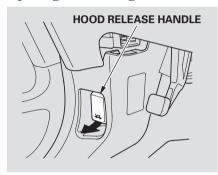
1. Park the vehicle, and set the parking brake. Pull the hood release handle located under the lower left corner of the dashboard. The hood will pop up slightly.
