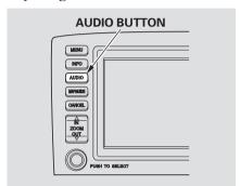
To adjust the sound, push the AUDIO button, then enter the sound grid by touching the SOUND icon on the display.
