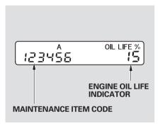
When the vehicle needs maintenance, maintenance codes appear on the information display.
