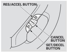
Cruise control may not hold the set speed when you are going up and down hills. If your speed increases going down a hill, use the brakes to slow down. This will cancel cruise control. To resume the set speed, press the RES/ACCEL button. The indicator on the instrument panel will come back on.
