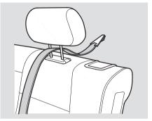
1. After properly securing the child seat (see page 49), lift the head restraint, then route the tether strap over the seat-back and through the head restraint legs.
