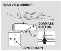
The direction and center position icons come on when you turn the ignition switch to the ON (II) position. The system then begins to check the vehicle direction and illuminates the appropriate icon(s).
