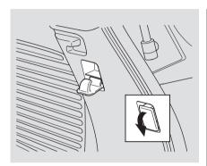
The hooks on each side of the tailgate and on the underside of the cargo area storage compartment lid are for plastic grocery bags. To use the hook on the storage compartment lid, open the lid, and attach the cord to one of the shafts of the third seat center head restraint.
