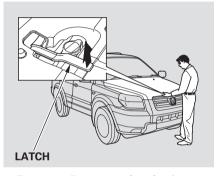
2. Put your fingers under the front edge of the hood near the center. Slide your hand to the left until you feel the hood latch handle. Push this handle up to release it. Lift up the hood.
