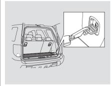
You can use the cargo net to secure items in the cargo area, and store small items between the two halves of the net. To install the cargo net, hook the loops on the four corners of the net to the tabs at both sides of the tailgate sill.
