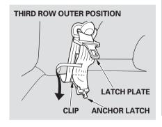
Pull out the anchor latch and the latch plate from each holding slot in the ceiling, and pull out the seat belt to extend it.
