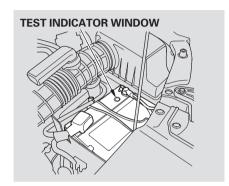
Check the condition of the battery monthly by looking at the test indicator window. The label on the battery explains the test indicator's colors. Check the terminals for corrosion (a white or yellowish powder). To remove it, cover the terminals with a solution of baking soda and water. It will bubble up and turn brown. When this stops, wash it off with plain water. Dry off the battery with a cloth or paper towel. Coat the terminals with grease to help prevent further corrosion.
