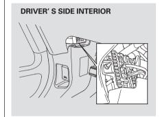
The vehicle's fuses are located in four fuse boxes. The interior fuse boxes are located under the dashboard on the driver's and passenger's side.
