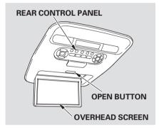
Open the overhead screen by pushing the OPEN button. The screen will swing down part-way. Pivot the screen the rest of the way. If you pivot the screen too far forward, past the second detent, the display will turn off. Pivot the screen back to the second or first detent to turn the display back on. To close the screen, pivot it up until it latches.
