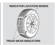
Your tires have wear indicators molded into the tread. When the tread wears down, you will see a band 1/2 inch (12.7 mm) wide band across the tread. This shows there is less than 1/16 inch (1.6 mm) of tread left on the tire.
