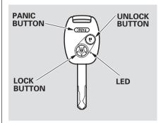
LOCK — Press this button once to lock all doors and the tailgate. Some exterior and interior lights will flash. When you push LOCK twice within 5 seconds, you will hear a beep to verify that the security system has set. You cannot lock it if any door is not fully closed or the key is in the ignition switch.
