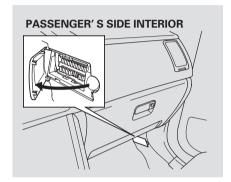
To open the passenger's side fuse box, pull the right edge of the cover.
