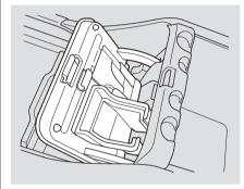
To open the console compartment, pull up on the lever, and lift the lid.
