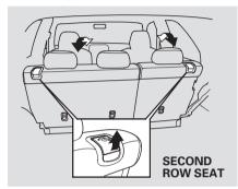
To change the angle of the seats in the second row seat-backs, pull up the handle on the seat-back. Moving the short vertical switch forward or backward adjusts the seat back in those directions.
