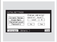
Select "Parental Level" by pressing the ▼ or ▲ button. You will see the submenu shown above. If you select "No," and press the ENT button, the display returns to the "Others" menu.
