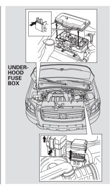
**Checking and Replacing Fuses**
