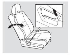
To change the seat-back angle of the front seat, pull up the lever on the outside of the seat bottom.
