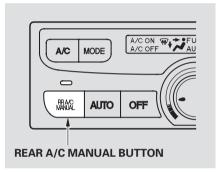
When the RR A/C MANUAL button is on, you can adjust the temperature of the rear passenger compartment manually from the second row seat.
