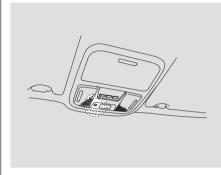
The courtesy light between the map lights comes on when you turn the parking lights on. To adjust its brightness, turn the Select/Reset knob on the instrument panel.
