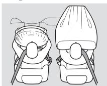
Your vehicle has a supplemental restraint system (SRS) with front airbags to help protect the heads and chests of the driver and a front seat passenger during a moderate to severe frontal collision (see page 28 for more information on how your front airbags work).
