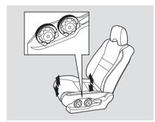
The height of your driver's seat is adjustable. Turn the front dial on the outside of the seat cushion to raise the front of the seat bottom, and turn the rear dial to raise the rear.
