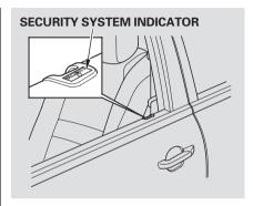
Once the security system is set, opening any door, the tailgate, or the hood without using the key or the remote transmitter, will cause it to alarm. It also alarms if the radio is removed from the dashboard or the wiring is cut.
