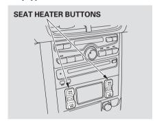
Both front seats are equipped with seat heaters. Because of the sensors for the side airbag system, there is no heater in the passenger's seatback. The ignition switch must be ON (II) to use the heaters.
