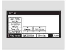
To do a chapter search, select "Chapter" by pressing the ▼ or ▲ button. Change the number on the right submenu by pressing the ▼ or ▲ button, and press the ENT button to begin the chapter search. If you press the RETURN button, the display returns to the play mode setup menu without doing the search.
