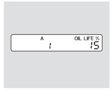
3. Press the Select/Reset knob for more than 10 seconds. The engine oil life and the maintenance item code(s) will blink.
