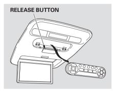
The rear control panel can be detached from the ceiling unit and used as a remote control. To remove it from the ceiling unit, press the release button. The control panel will swing down partway. Pivot it down further past the detent until it detaches from the hinge. To reinstall it, reverse the procedure.
