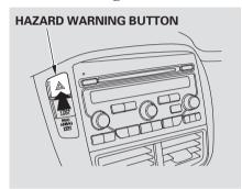
Push the red button to turn on the hazard warning lights (four-way flashers). This causes all four outside turn signals and both turn indicators in the instrument panel to flash. Use the hazard warning lights if you need to park in a dangerous area near heavy traffic, or if your vehicle is disabled.
