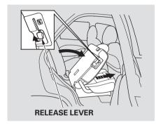
To get into the third row seats, pull up the lever on the side of the passenger's side second row seatback. The seat-back will tilt forward, and the seat will slide forward.
