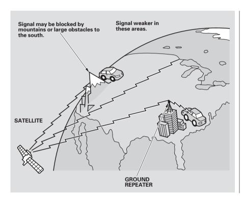
The XM satellites are in orbit over the equator; therefore, objects south of the vehicle may cause satellite reception interruptions. To help compensate for this, ground-based repeaters are placed in major metropolitan areas.
