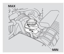
The fluid level should be between the MIN and MAX marks on the side of the reservoir. If the level is at or below the MIN mark, your brake system needs attention. Have the brake system inspected for leaks or worn brake pads.
