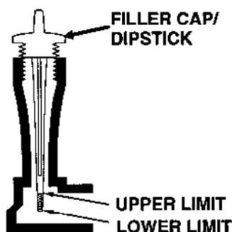
4. After checking the engine oil level, screw in the filler cap/dipstick securely.
