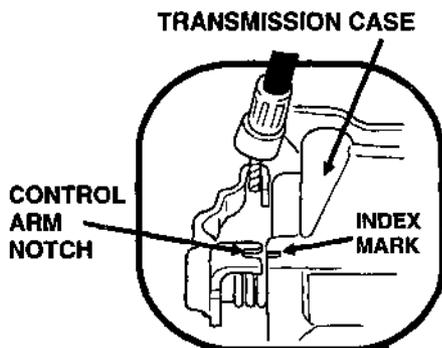
6. If adjustment is necessary, loosen the drive clutch cable lock nuts with a 10 mm wrench, and move the adjuster up or down as required. Tighten the lock nuts. Operate the clutch lever several times, and recheck control arm alignment.
