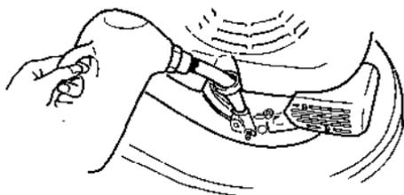
4. Fill with the recommended oil. Do not overfill; measure the oil level as shown on page 50.
