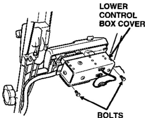
2. Remove the lower control box cover, and check the fuse. If it is burnt out, install the spare 1 ampere fuse provided with the mower.
