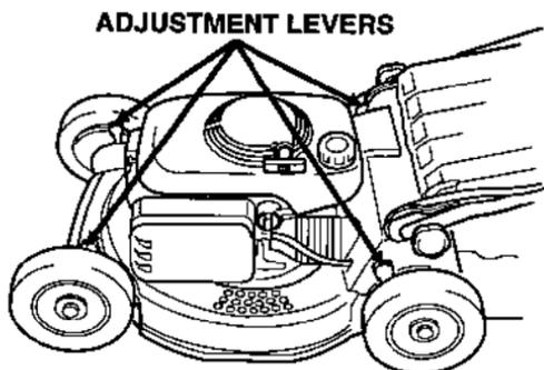
To adjust cutting height, pull each adjustment lever toward the wheel, and move it into another notch.
