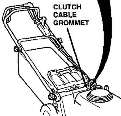
7. After the control arm is precisely aligned, start the engine and operate the drive clutch lever. Check to be sure the drive clutch lever operates properly.
