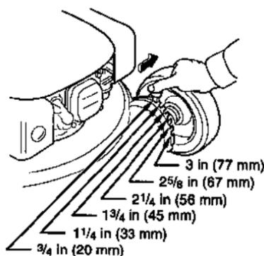
If you are not sure what cutting height to select, start with a high setting, and check the appearance of the lawn after mowing a small area. Then readjust cutting height if necessary.
