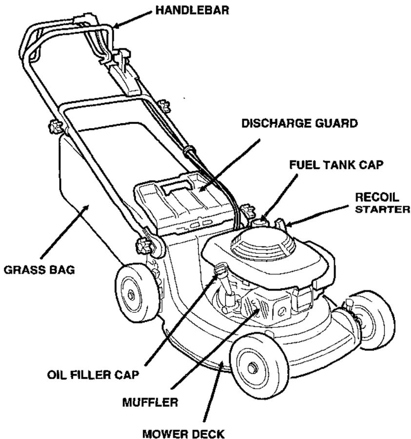
HR215K1HMA: Manual & electric starting; self-propelled; hydrostatic transmission
