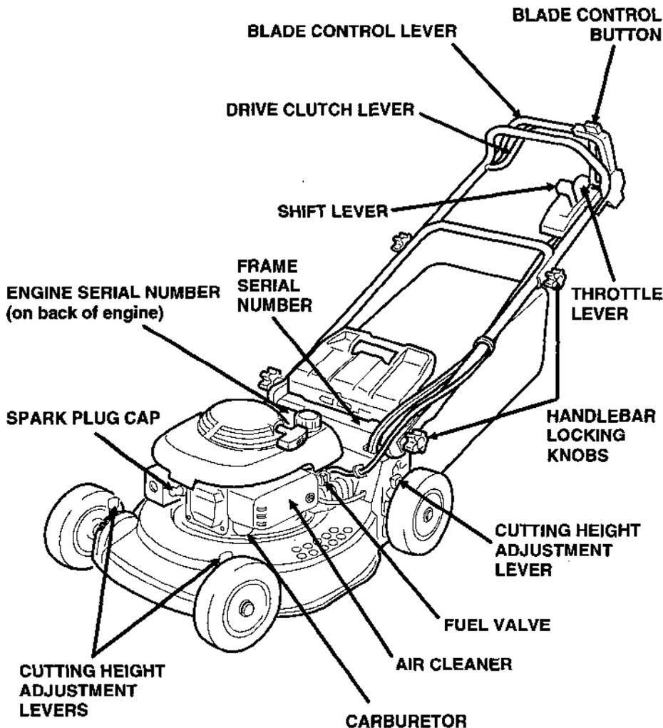
Record the frame and engine serial numbers in the space below. You will need these serial numbers when ordering parts and when making technical or warranty inquiries (see page 85).
