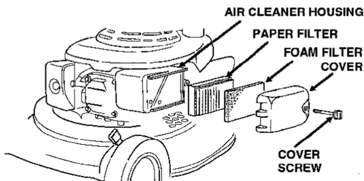
1. Unscrew and remove the air cleaner housing cover screw, then remove the air cleaner housing cover.
