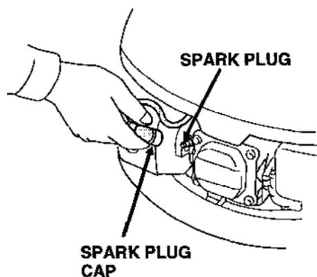
2. Remove the spark plug with a  $\frac{13}{16}$  in (21 mm) spark plug wrench.
