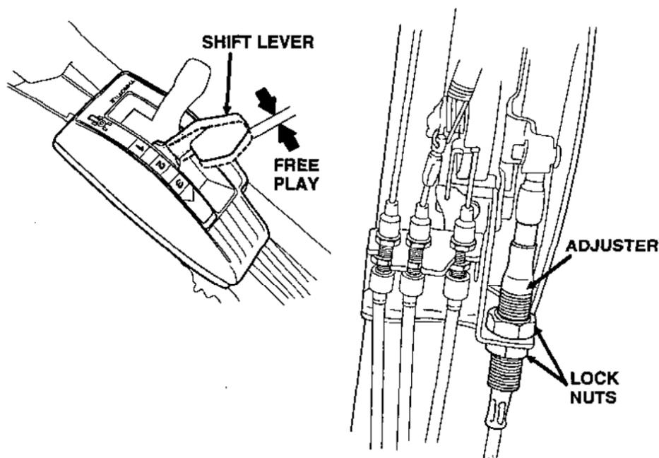
**Drive Clutch Cable Adjustment (HMA, HXA)**
