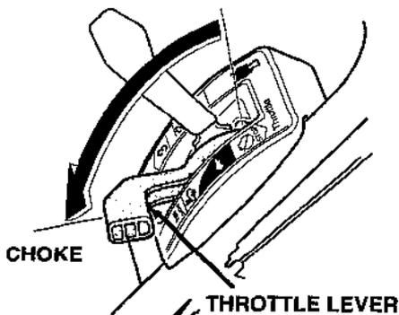
2. Move the throttle lever to the **FAST** position. The choke arm should move clockwise, until it contacts the stop post on the carburetor.
