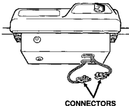
4. After the battery has been charged, disconnect the charger, and reconnect the battery connectors under the engine switch housing.
