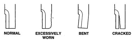
A dull blade can be sharpened, but a blade that is worn out, bent, cracked, or otherwise damaged must be replaced. A worn or damaged blade can break, causing blade pieces to be thrown from the mower.
