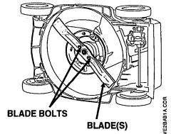
Inspect the blade(s) for wear and damage.
