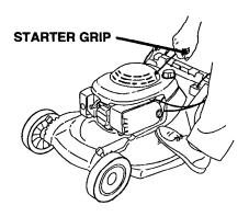
Move the throttle lever away from the CHOKE position as soon as the engine warms up enough to run smoothly without use of the choke. Set the throttle lever at FAST to mow or at SLOW to idle.
