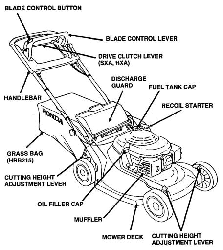
HRB215PXA: Manually propelled, high-lift blade, and grass bag.
