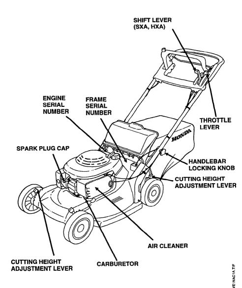
Record the frame and engine serial numbers in the space below. You will need these serial numbers when ordering parts and when making technical or warranty inquiries (see page 81).
