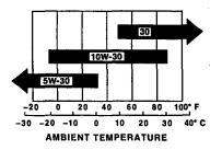
Use 4-stroke motor oil that meets or exceeds the requirements for API service classification SF, SG, or equivalent. Always check the API SERVICE label on the oil container to be sure it includes the
