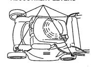
To adjust cutting height, pull each adjustment lever toward the wheel, and move it into another notch.
