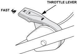
When you need to leave the mower for any reason, move the throttle to SLOW, then turn the engine OFF by releasing the flywheel brake lever.
