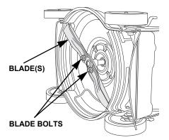
3. Inspect the blade(s) for wear and damage.
