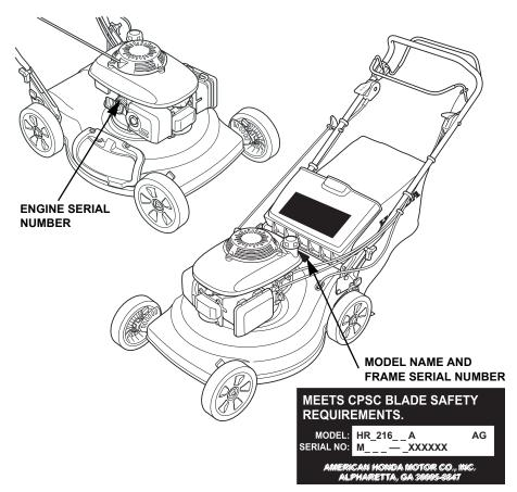
There are two serial numbers, one for the mower frame and one for the engine. Record the frame and engine serial numbers in the space below. You will need these serial numbers when ordering parts and when making technical or warranty inquiries (page 65).
