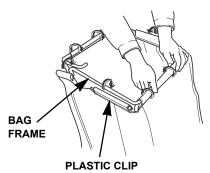
Lift the rear discharge guard, remove the mulching plug, then install the grass bag.
