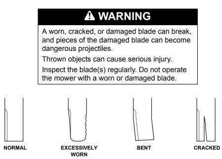
A dull blade can be sharpened, but a blade that is worn out, bent, cracked, or otherwise damaged must be replaced. A worn or damaged blade can break, causing blade pieces to be thrown from the mower. When a blade needs sharpening or replacement take the lawn mower to an authorized Honda servicing dealer. Or, if you have a torque wrench, you can remove and install the blade(s) yourself (page 32). Check that the blade bolts are tight (page 33).
