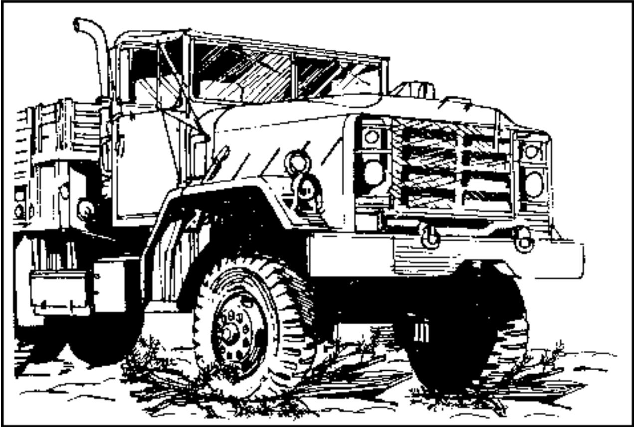
**Figure 3-2. Place material under tires to prevent freezing**
