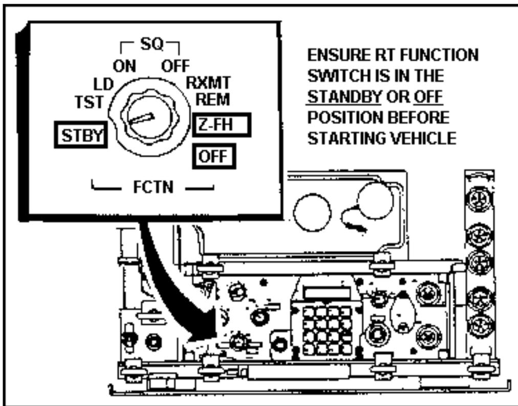
Figure 3-1. Protect radios when starting vehicles
