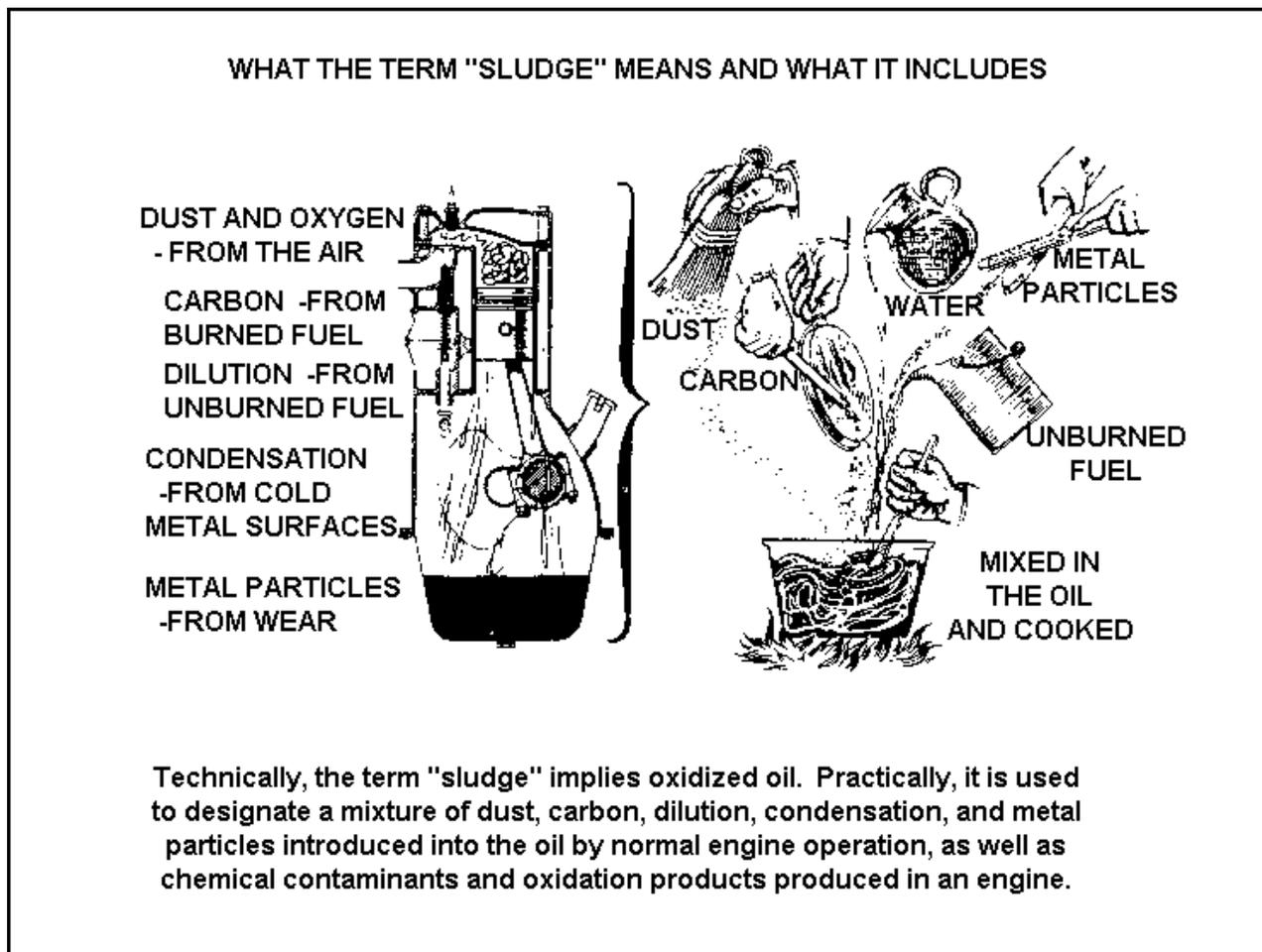
**Figure 3-3. Engine sludge**
