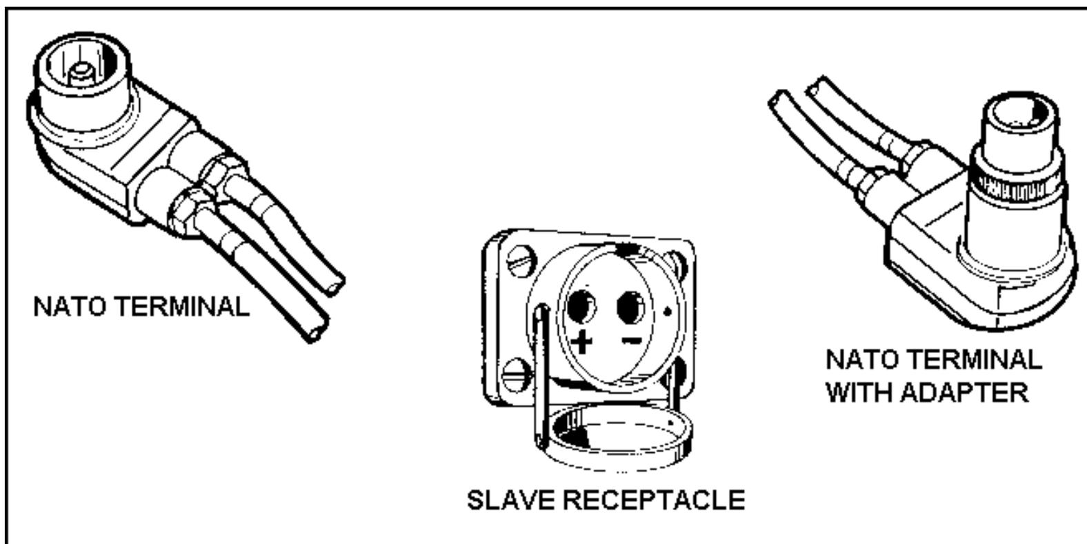
**Figure 1-8. Auxiliary power (slave) receptacle and terminals**
