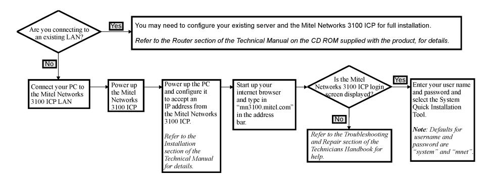
Note: On power up, the LED lights red. Once diagnostics are running the LED changes to amber. When diagnostics are complete and system is booting, the LED flashes green. Once this is complete, the LED lights solid green. If the LED remains red then refer to the Troubleshooting and Repair section of the Technicians Handbook.
