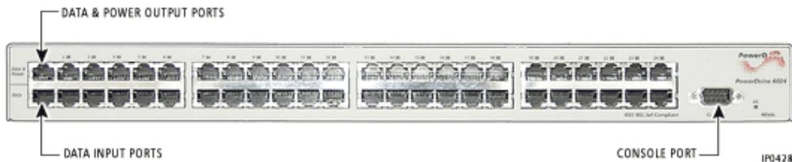
**10/100BASE-TX Data Input Ports, Lower 24 Ports**
