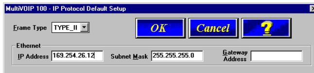
The default **Frame Type** is **TYPE\_II**. If this does not match your IP network, change the Frame Type by selecting SNAP from the **Frame Type** list. The available Frame Type choices are **TYPE\_II** and **SNAP**.
