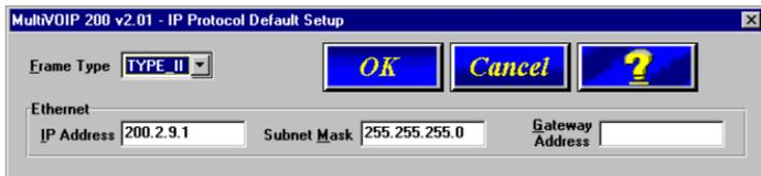
The default **Frame Type** is **TYPE\_II**. If this does not match your IP network, change the Frame Type by clicking the drop-down arrow and selecting SNAP. The available Frame Type choices are **TYPE\_II** and **SNAP**.
