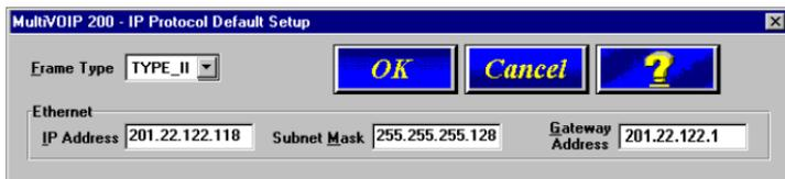
The default **Frame Type** is **TYPE\_II**. If this does not match your IP network, change the Frame Type by clicking the drop-down arrow and selecting SNAP. The available Frame Type choices are **TYPE\_II** and **SNAP**.
