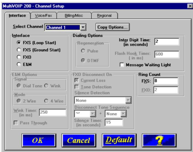
Configure each channel for the type of interface you are connecting to. The Interface tab defaults to **Channel 1** in the **Select Channel** field. To change the channel number, click the drop-down arrow and the list of channels is displayed. Highlight the channel you want to configure.
