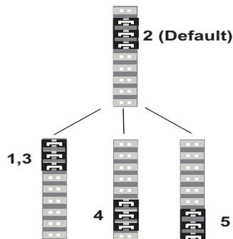
5. Change the jumper position for each voice/fax channel that is connecting to an E&M trunk that is not a type 2. If you have two voice/fax channel boards in your unit and you need to change the jumpers on the second board, remove the six screws from the top board and disconnect the ribbon cable from the top board.
