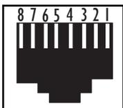
ATT-T568B (Cables wired pin-to-pin)
