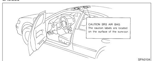
Caution and warning labels about the air bag system are placed in the vehicle.
