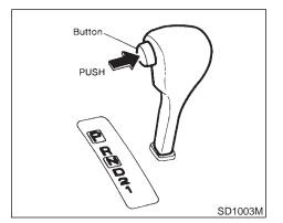
Push the button to shift into "P", "R" or from "D" to "2". All other positions can be selected without pushing the button.
