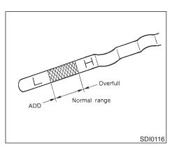
Remove the dipstick again and check the oil level. It should be between the "H" and "L" marks. If the oil level is below the "L" mark, remove the oil filler cap and pour recommended oil through the opening. Do not overfill.
