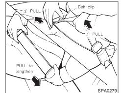
To lengthen, hold the tongue at a right angle to the belt and pull on the belt. To shorten, pull the end of the belt attached to the belt clip away from the tongue, and then pull the belt clip to take up the slack.
