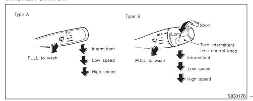
The windshield wiper and washer operates when the ignition key is in the "ACC" or "ON" position.
