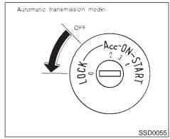
On automatic transmission models, the ignition lock is designed so that the key cannot be turned to "LOCK" and removed until the shift lever is moved to the "P" position.
