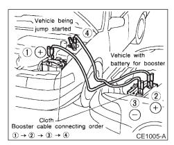
Always follow the instructions below. Failure to do so could result in damage to the charging system and cause personal injury.
