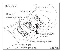
The power window only operates when the ignition key is in the "ON" position.
