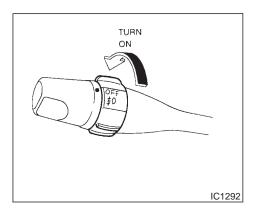
To turn the fog lights on, turn the headlight switch to the "  $\not\equiv$  " position, then turn the switch to the "  $\not\equiv$  " position. To turn them off, turn the switch to the "OFF" position.
