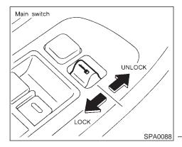
Operating the lock-unlock switch will lock or unlock all doors.
