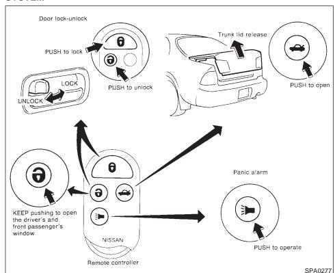
It is possible to lock/unlock all doors, to open the driver's and front passenger's windows, to release the trunk lid and to turn on or off the interior light by using the remote controller from outside the car.
