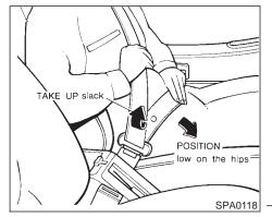
Slowly pull the seat belt out of the retractor and insert the tongue into the buckle until it snaps.
