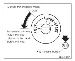
The switch includes an anti-theft steering lock device.
