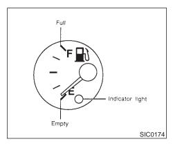
The indicator light comes on when the fuel tank is getting low. Refuel as soon as it is convenient, preferably before the gauge reaches "E". There should be a small reserve of fuel in the tank when the fuel gauge needle reaches "E".
