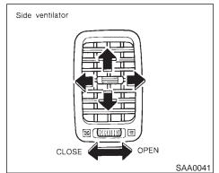
Open or close, and adjust the air flow direction of ventilators.
