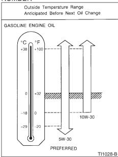
SAE 5W-30 viscosity oil is preferred for all temperatures. SAE 10W-30 viscosity oil may be used if the ambient temperature is above 0°F (-18°C).
