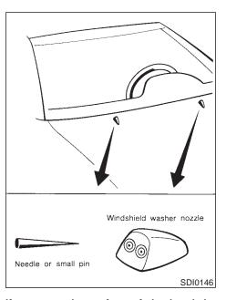
If you wax the surface of the hood, be careful not to let wax get into the washer nozzle. This may cause clogging or improper windshield washer operation. If wax gets into the nozzle, remove it with a needle or small pin.
