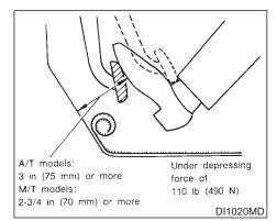
With the engine running, check the distance between the upper surface of the pedal and the metal floor. If it is out of the range shown above, see your NISSAN dealer.
