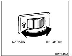
The instrument brightness control operates when the light switch is in the " ${\tt EDGE}$ " or " ${\tt gO}$ " position.
