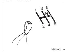
To change gears, fully depress the clutch pedal, then move the gearshift lever. After shifting, release the clutch slowly.
