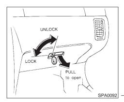
When locking or unlocking the glove box, use the master key.
