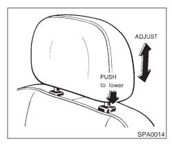
lower, push the lock knob and push the head restraint down.
