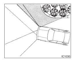
The cornering light provides additional illumination toward the turning direction. The light will come on when the turn signal lever is moved to the right or left with the headlights on.
