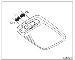
The interior light has a three-position switch.
