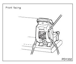
seat belt is allowed to wind back into the retractor, the automatic locking mode (child restraint mode) is canceled; the seat belt may be used as normal and will only lock during a sudden stop or impact.
