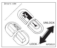
To lock from the outside without a key, push the door lock button (driver side only) or the door lock knob (driver or passenger side), then close the door. When locking the door this way, be certain not to leave the key inside the vehicle.
