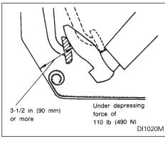
With the engine running, check the distance between the upper surface of the pedal and the metal floor. If it is out of the range shown above, see your NISSAN dealer.
