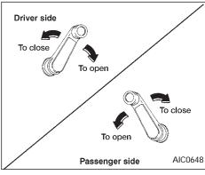
The side windows can be opened or closed by turning the hand crank on each door.
