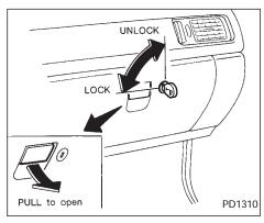
Use the master key to lock or unlock the glove box.
