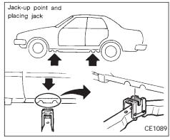
Jacking up and removing tire
