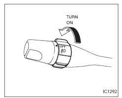
To turn the front fog lights on, rotate the switch to the  $\not\equiv \bigcirc$  position.
