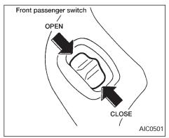
The front passenger switch operates only the front passenger window. To open or close the window, press and hold the switch.
