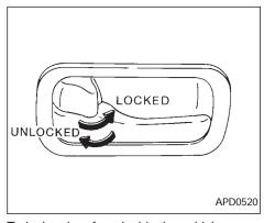
To lock a door from inside the vehicle, press the lock knob (located above the door handle) until it is flush with the door panel. To unlock, pull the lock knob to its outer position.
