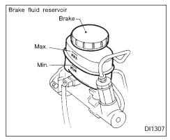
Check the brake fluid level in the reservoir. If the fluid level is below the MIN line or the brake warning light comes on, add **DOT 3** fluid up to the MAX line. If fluid must be added frequently, the system should be thoroughly checked by your NISSAN dealer.
