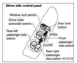
The power windows operate only when the ignition key is in the ON position. To open a window, press down on the switch. To close a window, push up on the switch. To stop the opening or closing function at any time, simply release the switch.
