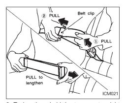
To lengthen, hold the tongue at a right angle to the belt and pull on the belt. To shorten, pull the end of the belt attached to the belt clip away from the tongue, then pull the belt clip to take up the slack.
