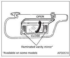
To access the vanity mirror, pull the sun visor down and flip open the mirror cover. Some vanity mirrors are illuminated and turn on when the mirror cover is opened.
