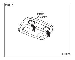
The light illuminates when the trunk lid is opened. When the trunk lid is closed, the light goes off.
