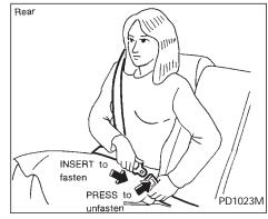
Slowly pull the seat belt out of the retractor and insert the tongue into the buckle until it snaps.
