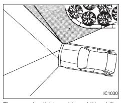
The cornering light provides additional illumination toward the turning direction. The light on the turning direction side comes on when a turn is signaled with the headlights on.
