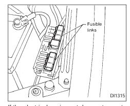
If the electrical equipment does not operate and fuses are in good condition, check the fusible links. If any of these fusible links are melted, replace only with genuine NISSAN parts.
