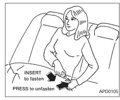
2-POINT TYPE WITHOUT RETRACTOR (center position of rear seat)
