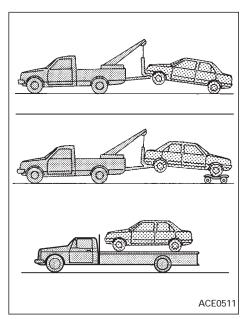
NISSAN recommends that your vehicle be towed with the driving (front) wheels off the ground as illustrated.
