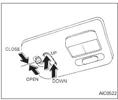
The sunroof only operates when the ignition key is in the ON position.
