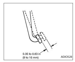
Press the pedal by hand and be sure the free travel is within the limits shown above. If free travel is out of the range shown above, see your NISSAN dealer.
