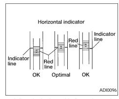
Adjust the horizontal indicator by turning the adjusting screw with a Phillips screwdriver.
