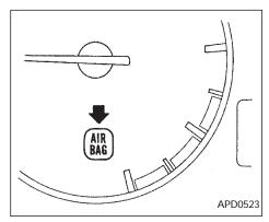
The supplemental air bag warning light, displaying AIR BAG in the instrument panel, monitors the circuits of the supplemental air bag. The circuits monitored by the supplemental air bag light are the diagnosis sensor unit, supplemental air bag modules and all related wiring.
