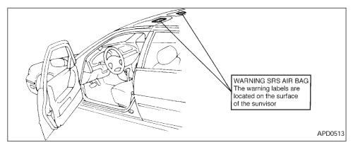
Warning labels about the supplemental air bag system are placed in the vehicle as shown in the illustration.
