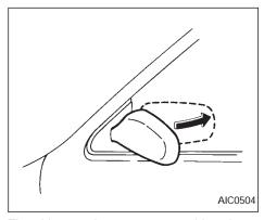
The driver and passenger outside mirrors are foldable. Push the outside mirror backward to fold it.
