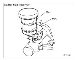
Check the clutch fluid level in the reservoir (manual transmission only). If the fluid level is below the MIN line, add **DOT 3** fluid up the MAX line. If fluid must be added frequently, the system should be thoroughly checked by your NISSAN dealer.
