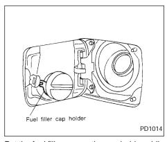
Put the fuel filler cap on the cap holder while refueling.
