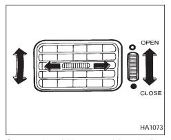
Open or close (side vents only), and adjust the air flow direction of ventilators.
