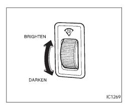
The instrument brightness control operates when the light switch is in the EDQE or Dosition.
