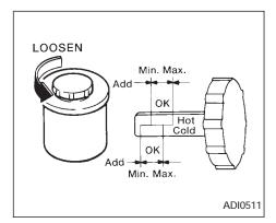
Check the fluid level in the reservoir.
