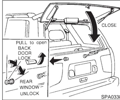
To open the rear window, turn the key fully clockwise and pull the opener handle. To close, lower and push the rear window down securely.
