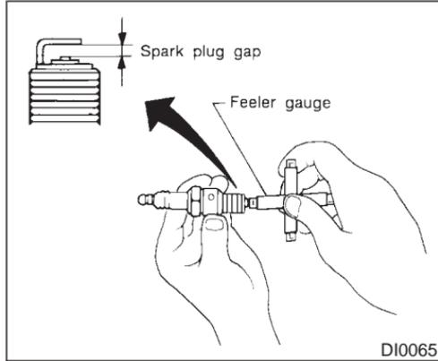
3. Check each new spark plug gap with a feeler gauge. Correct it as required.
