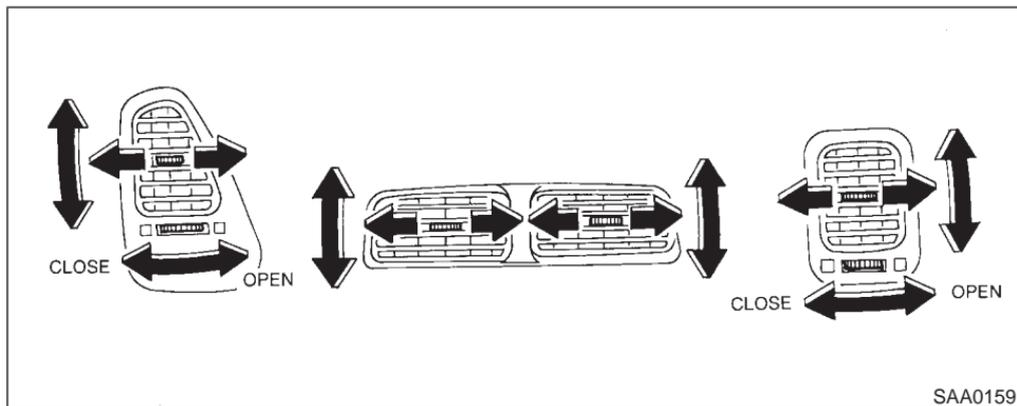
Open or close, and adjust the air flow direction of ventilators.
