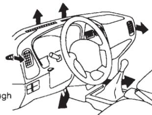
← : Air passed through heater core
