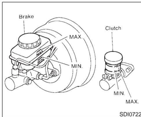
Check the fluid level in the reservoir. If the fluid level is below the MIN. line or the brake warning light comes on, add DOT 3 fluid up to the MAX. line.
