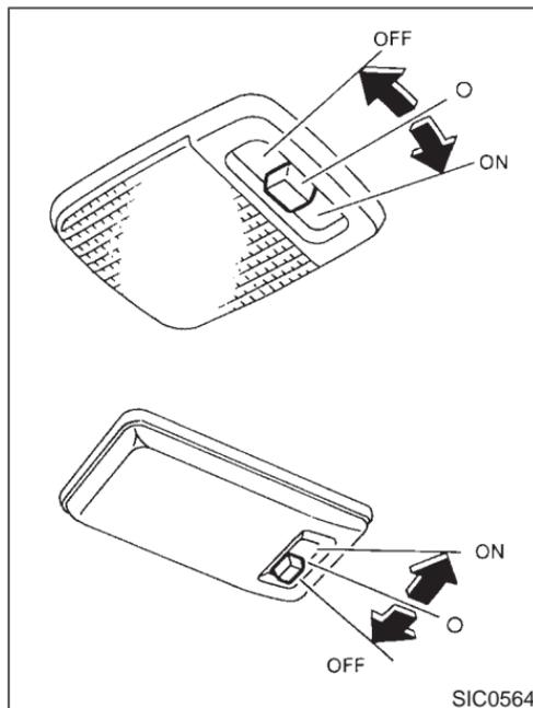
The interior light has a three position switch. The interior light will operate regardless of ignition key position.
