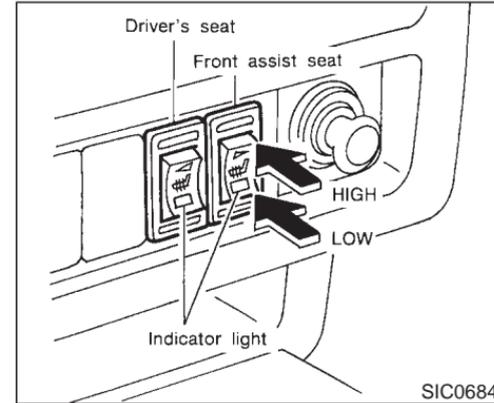
The front seat(s) are warmed by built-in heaters. The switches located on the instrument panel can be operated independently of each other.
