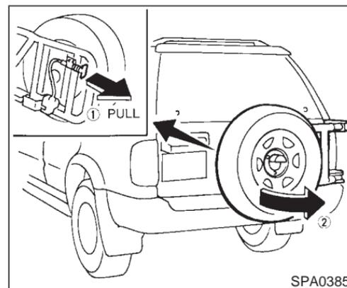
When opening the back door, first open the spare tire carrier in the sequence shown in the illustration above. Then insert the stopper into the hole to secure the carrier in the open position.
