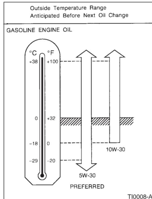
SAE 5W-30 viscosity oil is preferred for all temperatures. SAE 10W-30 viscosity oil may be used if the ambient temperature is above 0°F (-18°C).
