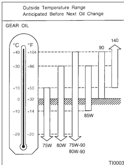
**75W-90 for transfer, and 80W-90 for differential are preferable if the ambient temperature is below 104°F (40°C).**
