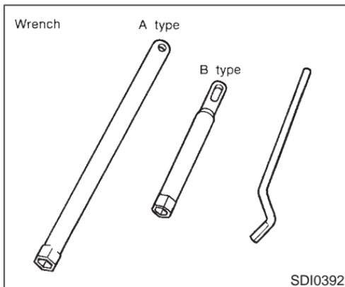
2. Remove spark plugs with a spark plug wrench. (Type A or B)
