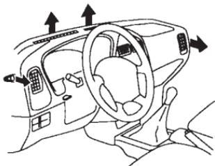
← : Air passed through heater core
