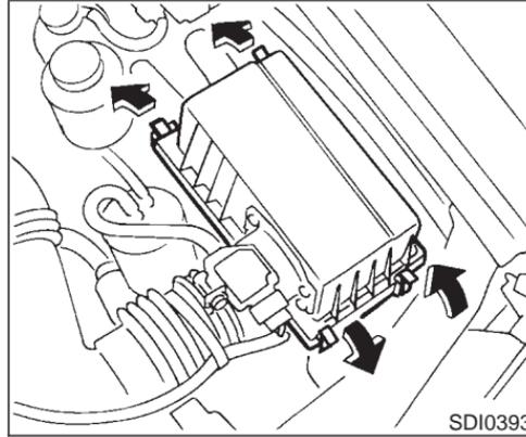
The filter element should not be cleaned and reused as it is given a special treatment. We recommend it be replaced according to the maintenance intervals. See "Periodic maintenance" in the "9. Maintenance" section for maintenance intervals. When replacing the filter, wipe the inside of the air cleaner housing and the cover with a damp cloth.
