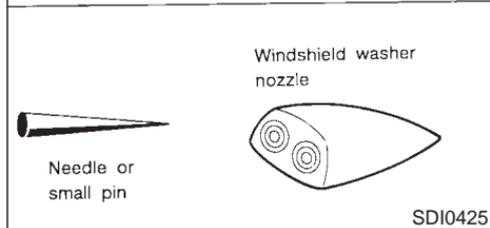
If you wax the surface of the hood, be careful not to let wax get into the washer nozzle. This may cause clogging or improper windshield washer operation. If wax gets into the nozzle, remove it with a needle or small pin.
