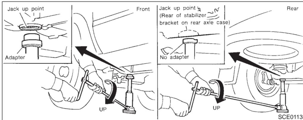
Jacking up the vehicle and removing the damaged tire
