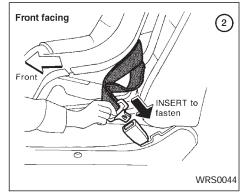
Route the seat belt tongue through the child restraint and insert it into the buckle until you hear and feel the latch engage.
