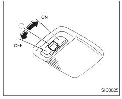
The interior light has a three-position switch.
