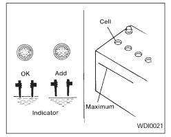
2. Check the fluid level in each cell.
