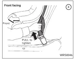
4. Allow the seat belt to retract slightly. Pull up on the seat belt to remove any slack in the belt.
