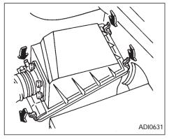
The air cleaner filter should not be cleaned and reused. Replace it according to the maintenance intervals shown in the "Maintenance" section of this manual. When replacing the filter, wipe the inside of the air cleaner housing and the cover with a damp cloth.
