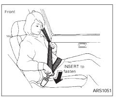
THREE-POINT TYPE SEAT BELT WITH RETRACTOR
