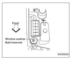
To fill the window washer fluid reservoir, lift the cap off the reservoir tank and pour the window washer fluid into the tank opening.
