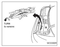
2. To remove the jack, turn the jack screw counterclockwise. Use the tapered end of the jack rod to loosen the jack from its storage position.
