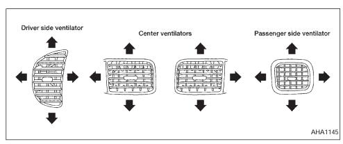
Adjust air flow direction by moving the ventilator slide.
