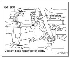
3. Flush the cooling system by running fresh water through the radiator.
