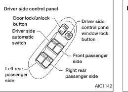
The power windows operate only when the ignition key is in the ON position.
