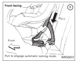
3. Pull on the shoulder belt until all of the belt is fully extended. At this time, the seat belt retractor is in the automatic locking mode (child restraint mode). It reverts back to emergency locking mode when the seat belt is fully retracted.
