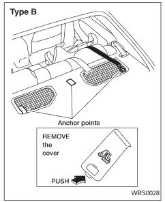
Remove the anchor cover from the anchor point which is located directly behind the child seat.
