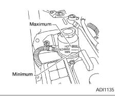
Check the fluid level in the reservoir.
