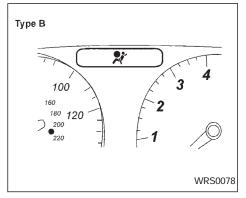
When the ignition key is in the ON or START position, the supplemental air bag warning light illuminates for about 7 seconds and then turns off. This means the system is operational.
