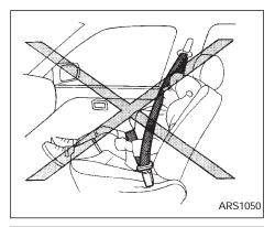
All seat belt assemblies including retractors and attaching hardware should be inspected after any collision by an authorized NISSAN dealer. NISSAN recommends that all seat belt assemblies in use during a collision be replaced unless the collision was minor and the belts show no damage and continue to operate properly. Seat belt assemblies not in use during a collision should also be inspected and replaced if either damage or improper operation is noted.
