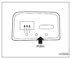
To defog the rear window glass, start the engine and push the rear window defogger switch on. (The indicator light on the switch comes on.) Push the switch again to turn the defogger off.
