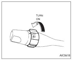
To turn the front fog lights on, rotate the switch to the  $\frac{1}{2}$  position.
