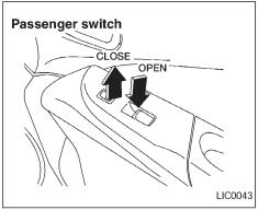
The passenger side switch opens or closes only the passenger side window. To open the window, push the switch down. To close the window, lift the switch up.
