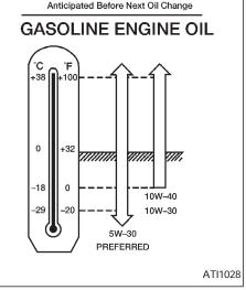
SAE 5W-30 viscosity oil is preferred for all temperatures. SAE 10W-30, SAE 10W-40 viscosity oils may be used if the ambient temperature is above 0°F (-18°C).
