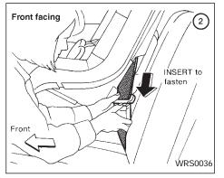
2. Route the seat belt tongue through the child restraint and insert it into the buckle until you hear and feel the latch engage.
