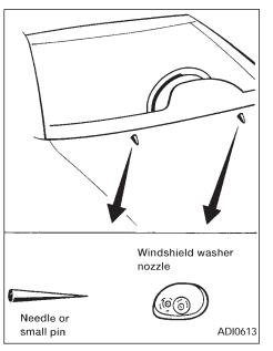
When you wax the surface of the hood, be careful not to let wax get into the washer nozzle. This may cause clogging or improper windshield washer operation. If wax gets into the nozzle, remove it with a needle or small pin.
