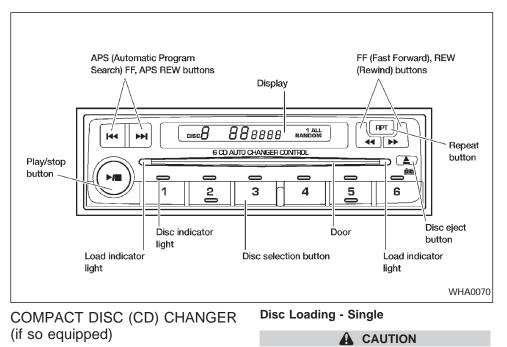
To use the CD changer, turn the ignition key to the ACC or ON position.
