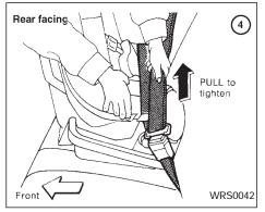
4. Allow the seat belt to retract. Pull up on the seat belt to remove any slack in the belt.
