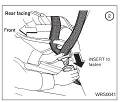
2. Route the seat belt tongue through the child restraint and insert it into the buckle until you hear and feel the latch engage.
