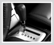
**NOTE:** With the transmission in the B (Brake) position and your foot off the accelerator pedal, engine braking will be applied.
