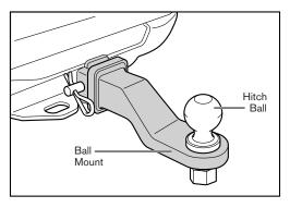
shank diameter and weight rating for the ball mount as well as the coupler on your trailer. Using a  $1^{7}/_{8}$ " hitch ball in a 2" coupler, for example, could result in the trailer separating
