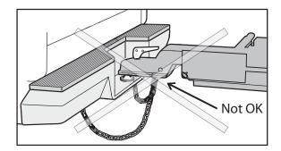
to the bumper and chains/cables when making a sharp turn, do not attach the chains/cables too close to the coupler. Consult your trailer manufacturer for the proper location of the chain/cable attachment to the trailer.
