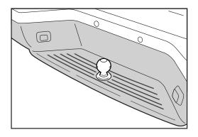
**Receiver Hitch** – A receiver hitch is bolted directly to the vehicle structure for added strength and durability. Nissan bolt-on receiver hitches are designed specifically for Nissan vehicles and include the necessary reinforcements, with ample clearance around bumpers, frame members, etc. These hitches allow for the removal of the ball mount when not towing.
