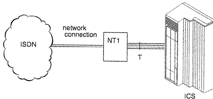
An S/T or T loop can be used in combination with an S loop to provide D-packet service for a point-of-sale terminal adapter (POSTA) or other D-packet device. D-packet service is a 16 kbps data transmission service that uses the D-channel of an ISDN line.
