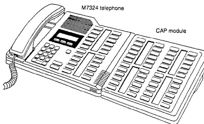
A CAP module is an add-on device that provides 48 extra memory or line buttons. You can connect one Norstar CAP module to the telephone to increase the number of lines it can handle.
