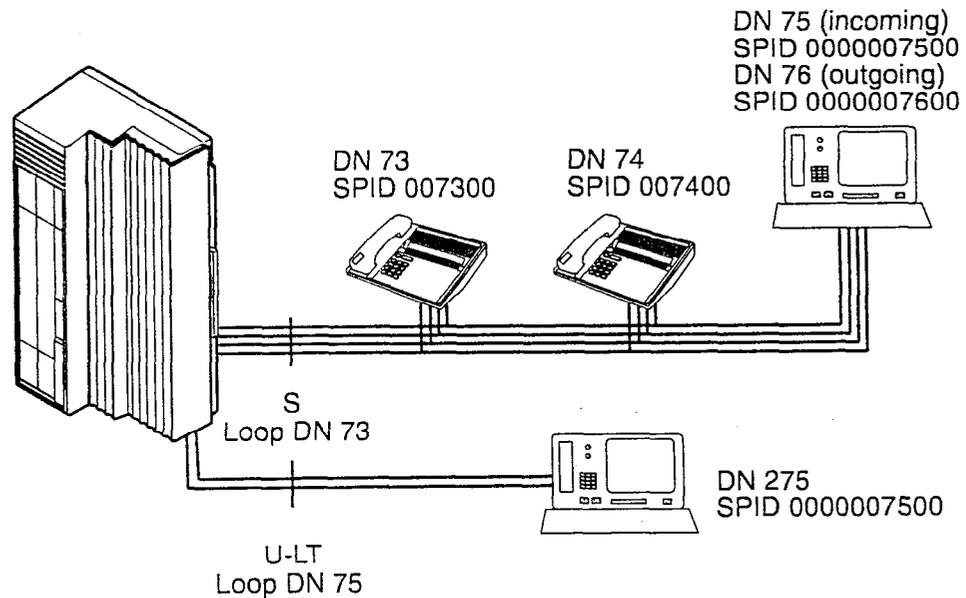
The following table uses the example in the illustration to show the Hardware programming for the S loop.
