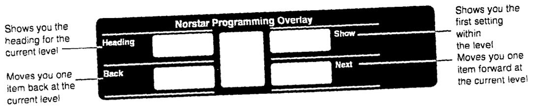
Programming buttons are active or inactive at different stages of programming. A button is active (meaning you can use that option), when the indicator next to it is lit (◀ or ▶).
