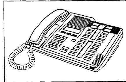
The indicators (▶) on the M7310 or M7324 telephone show which buttons can be used at that programming step. The functions on these buttons allow you to move through the headings and subheadings of Norstar programming.
