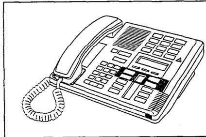
**M7324 telephone with a programming overlay**
