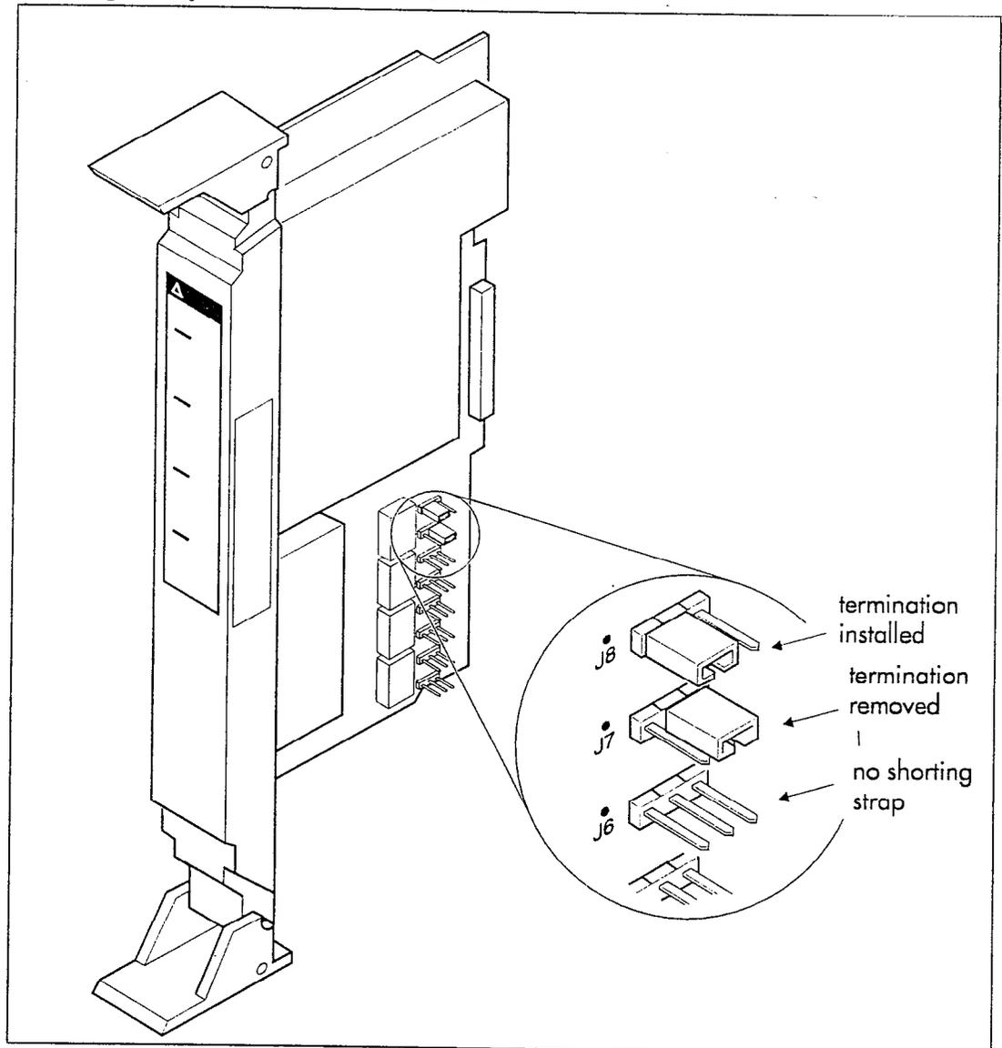
Make sure the shorting straps are installed on both the receive and transmit jumpers for the loop (see illustration). The jumpers are numbered top to bottom, but the loops associated with each pair of jumpers does not follow the same top-to-bottom sequence (see table).
