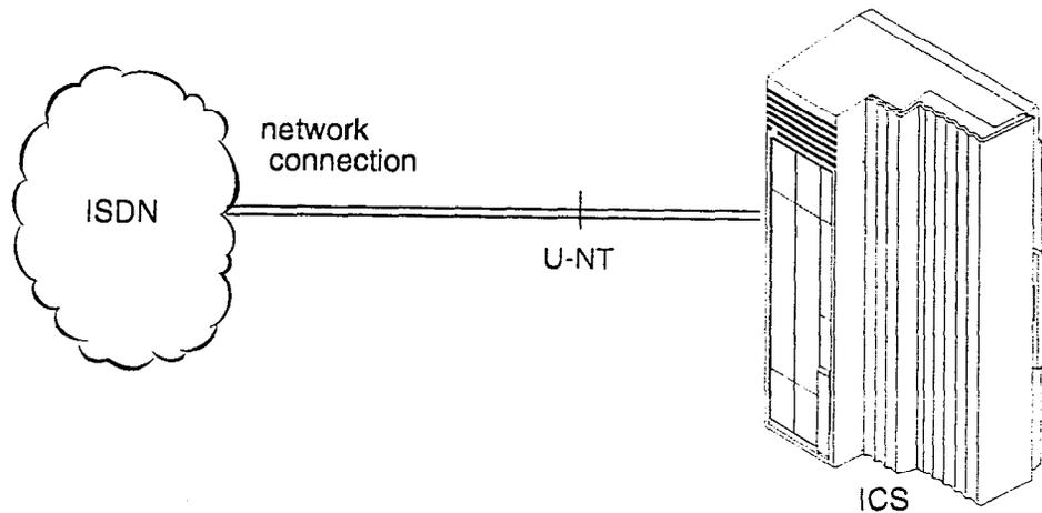
U-NT and U-LT loops can be used in combination to provide D-packet service for a point-of-sale terminal adapter (POSTA) or other D-packet device. D-packet service is a 16 kbps data transmission service that uses the D-channel of an ISDN line.
