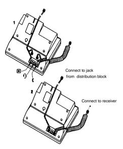
**ATTENTION** Before attempting to carry out <u>any</u> work on the telephone, ensure that the line cord is unplugged from the wall socket.
