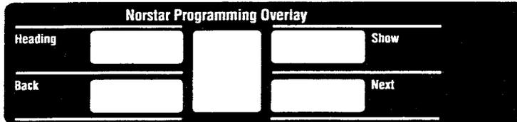
Place the programming overlay across the top four memory buttons of an M7310 or M7324 telephone.
