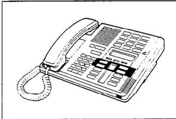
**M7324 telephone with a programming overlay**
