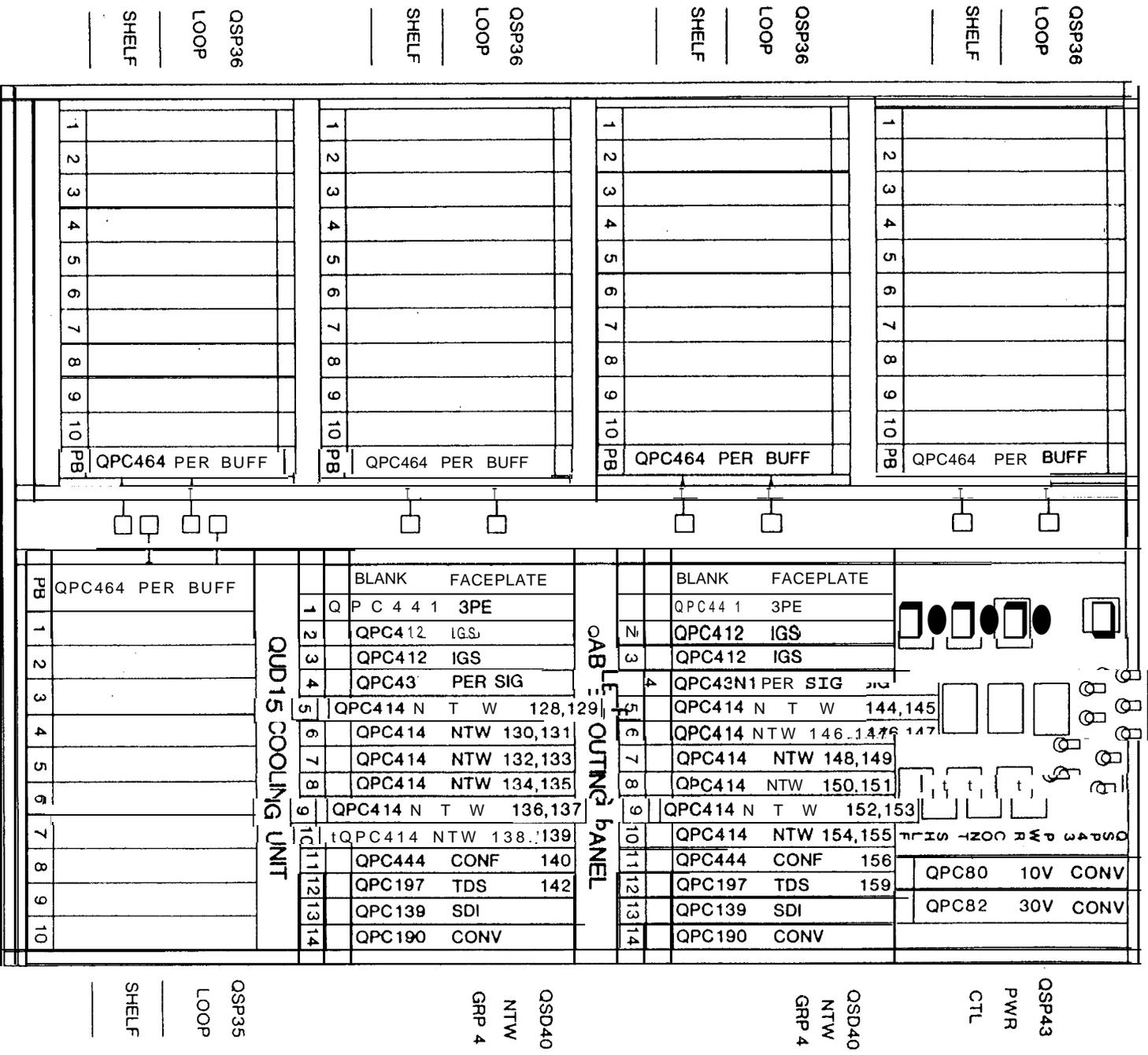
FIGURE 5-29: MERIDIAN SL-1XN QCA108 CABINET - REAR VIEW
