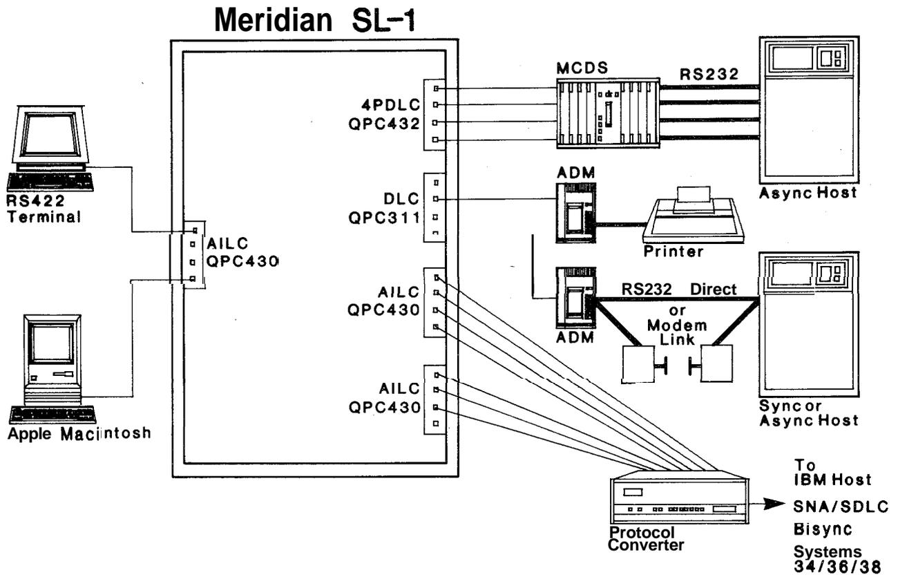
FIGURE 8-9: RS422 TERMINAL / MACINTOSH CONNECTION
