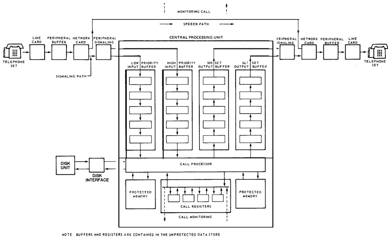
***A register is associated with and maintained throughout each call. The call register is a block of unprotected data, which holds transient information relative to the call***
