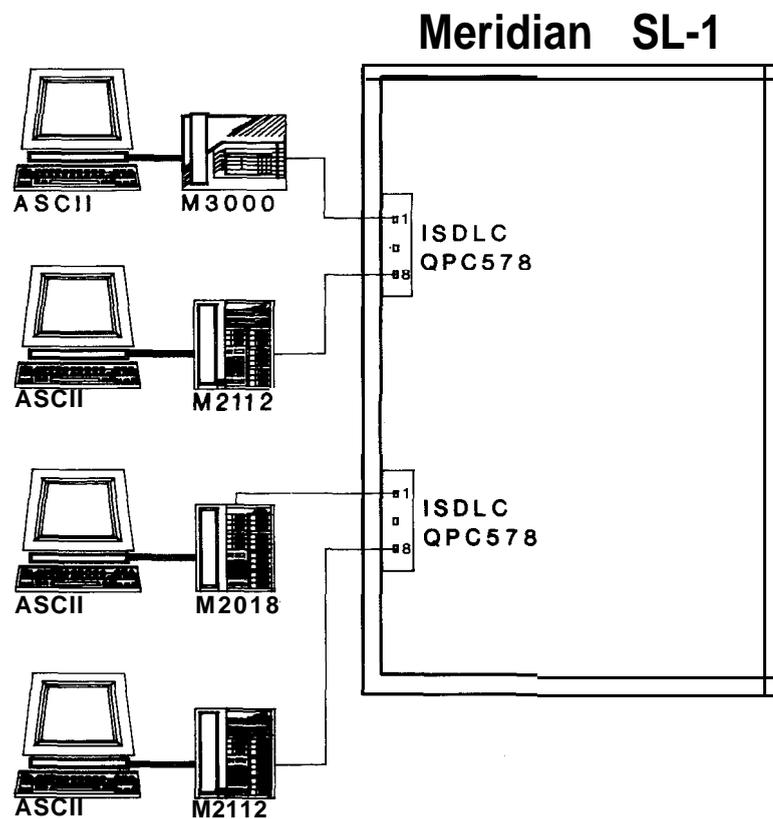
FIGURE 8-30: INTEGRATED SERVICES DIGITAL LINE CARD
