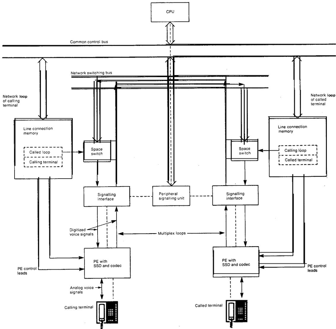
*This illustration shows how a call is set up on the Meridian SL-1. When a user lifts the handset to make a call, an SSD in the PE detects a change of state in the terminal. Under control of the peripheral signaling device, a message is sent to the CPU indicating that*
