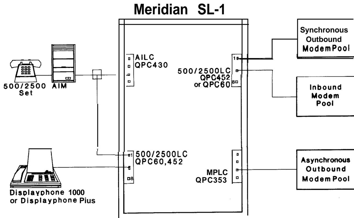
FIGURE 8-36: MODEM POOLING
