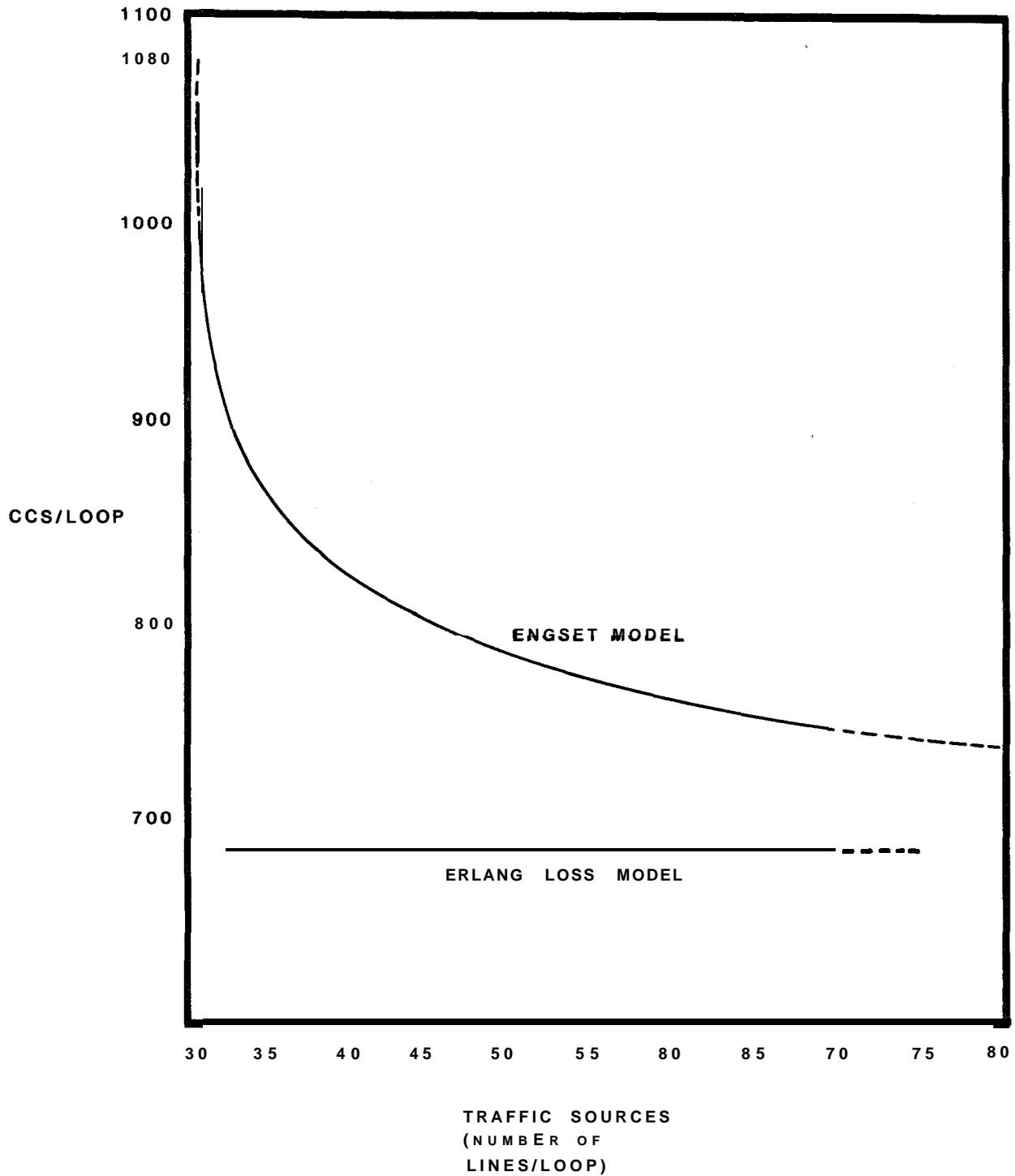
FIGURE 7-4: LOOP CAPACITY AS A FUNCTION OF TRAFFIC SOURCES
