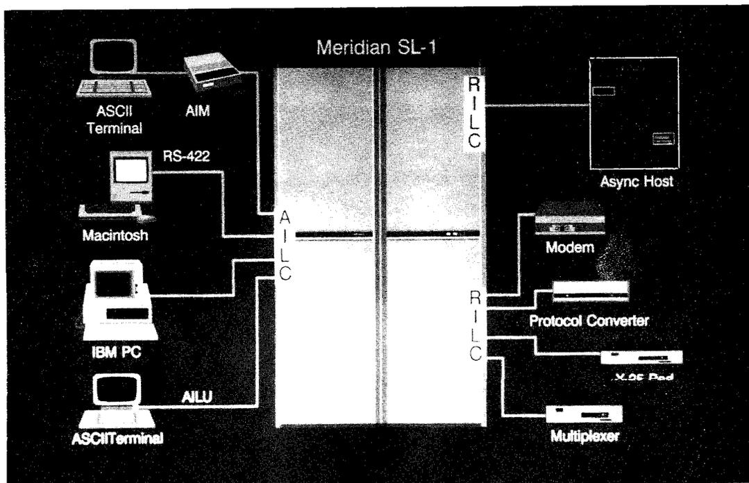
FIGURE S-34: RS-232C INTERFACE LINE CARD
