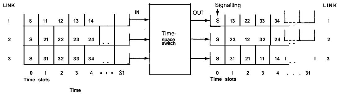
**With time-space switching, a conversation occupying any time slot on any inlet link can be switched to any time slot on any outlet link. For example, the conversation in time slot 1 on**
