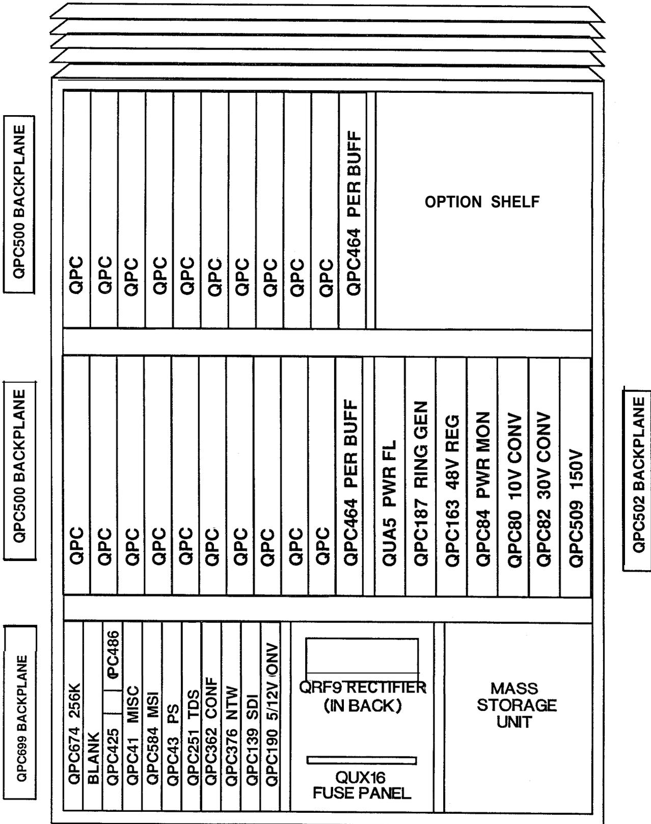
FIGURE510: MERIDIAN SL-1S QCA60 CABINET LAYOUT
