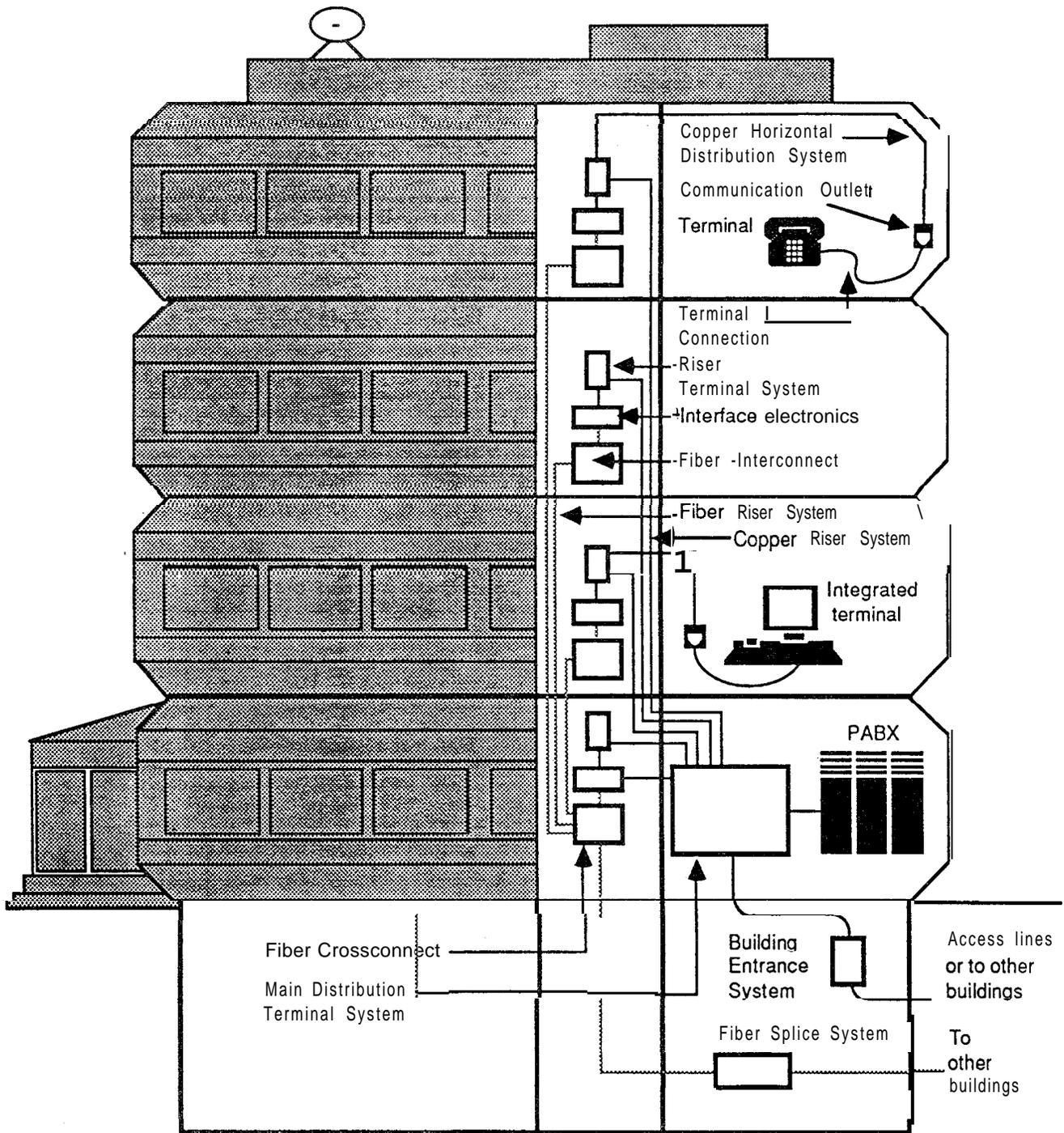
FIGURE 4- 11: INTEGRATED BUILDING DISTRIBUTION NETWORK
