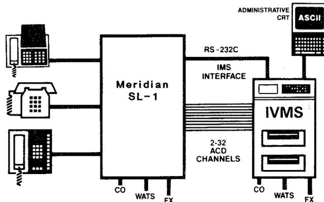
***The Integrated Voice Messaging System (IVMS) illustrates once again the versatility of the Meridian SL-1. An auxiliary processor interacts with the latter to provide sophisticated voice messaging capabilities to the user.***
