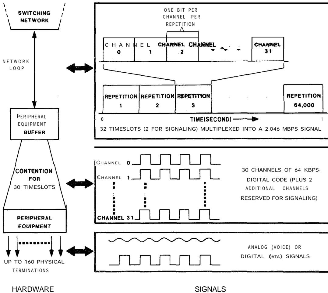
*This figure illustrates the principle of time division multiplexing as used in the multiplexed loops. Thirty-two digital signals are sent over a common path by transmitting them sequentially at different instants of time. As a result of eight-bit PCM*
