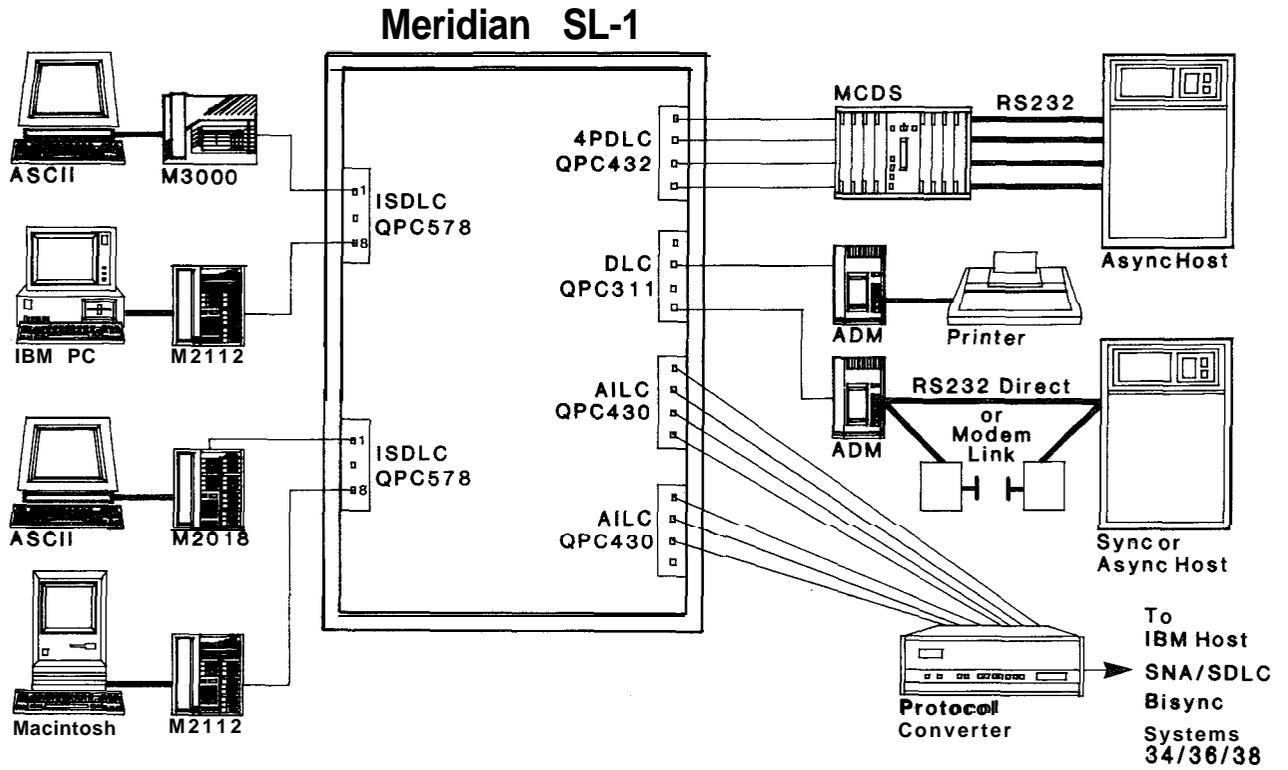
FIGURE 8-2: DIGITAL TELEPHONES WITH ASYNCHRONOUS DATA OPTION
