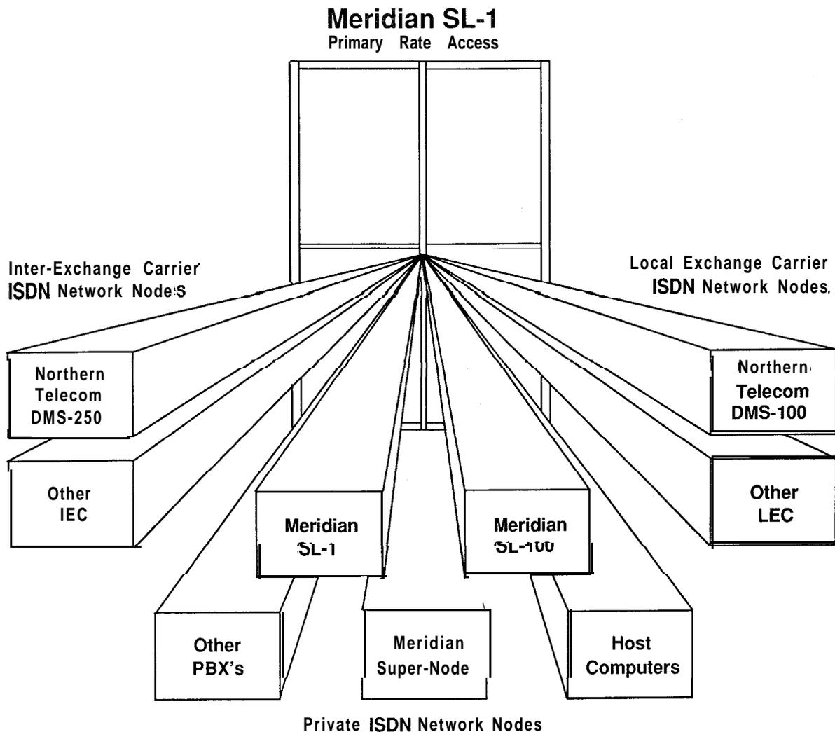
*Meridian SL-1 ISDN Primary Rate Access provides a 1544 Mbps (23B + D Channels) link to Local Exchange Carriers, Inter-Exchange Carriers or Private Network nodes.*
