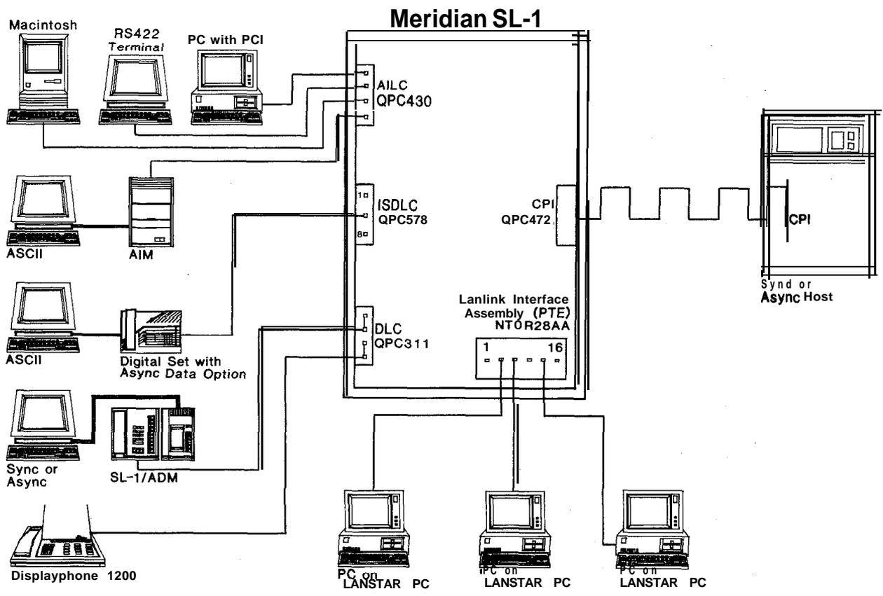
FIGURE 8-14: COMPUTER-TO-PBX INTERFACE
