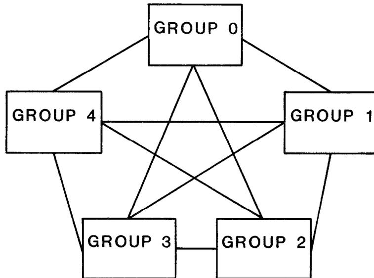
*In the multi-group arrangement, junctors provide an additional switching stage to extend the originating and terminating network loops from any one group to any other. Five network groups may be interconnected to constitute the capacity of the digital switching matrix.*
