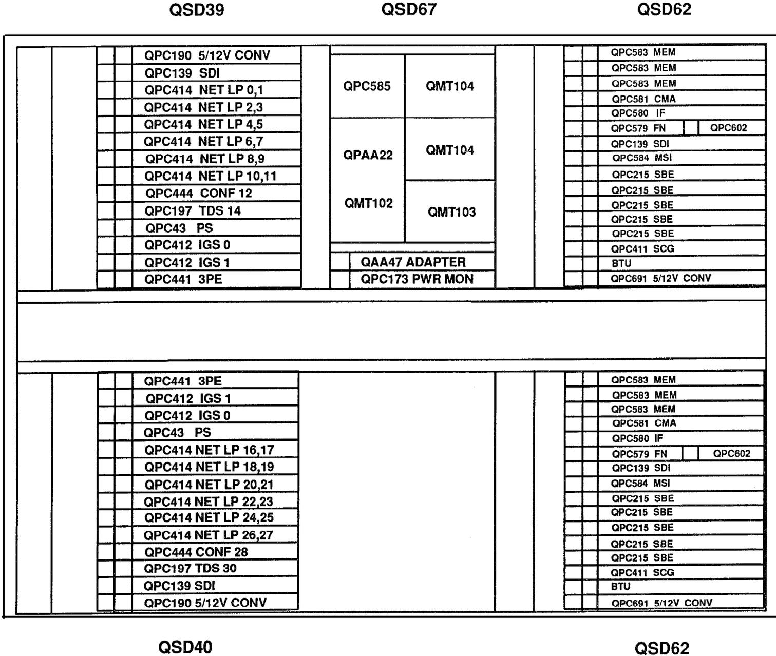
FIGURE 5-42: MERIDIAN SL-1XT QCA108 CABINET - FRONT VIEW
