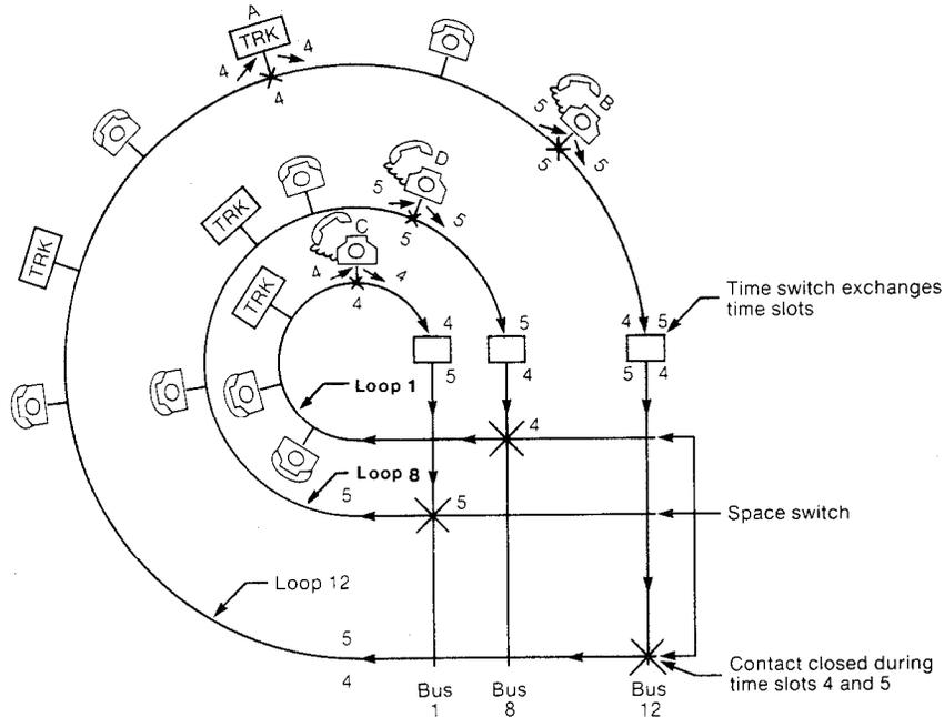
**Meridian SL-1 uses the simple space switch to route calls over its network. However, since the conversations are sampled and placed into time slots, new connections are made for every time slot instead of lasting for the duration of the conversation. There are 32 time slots in each**
