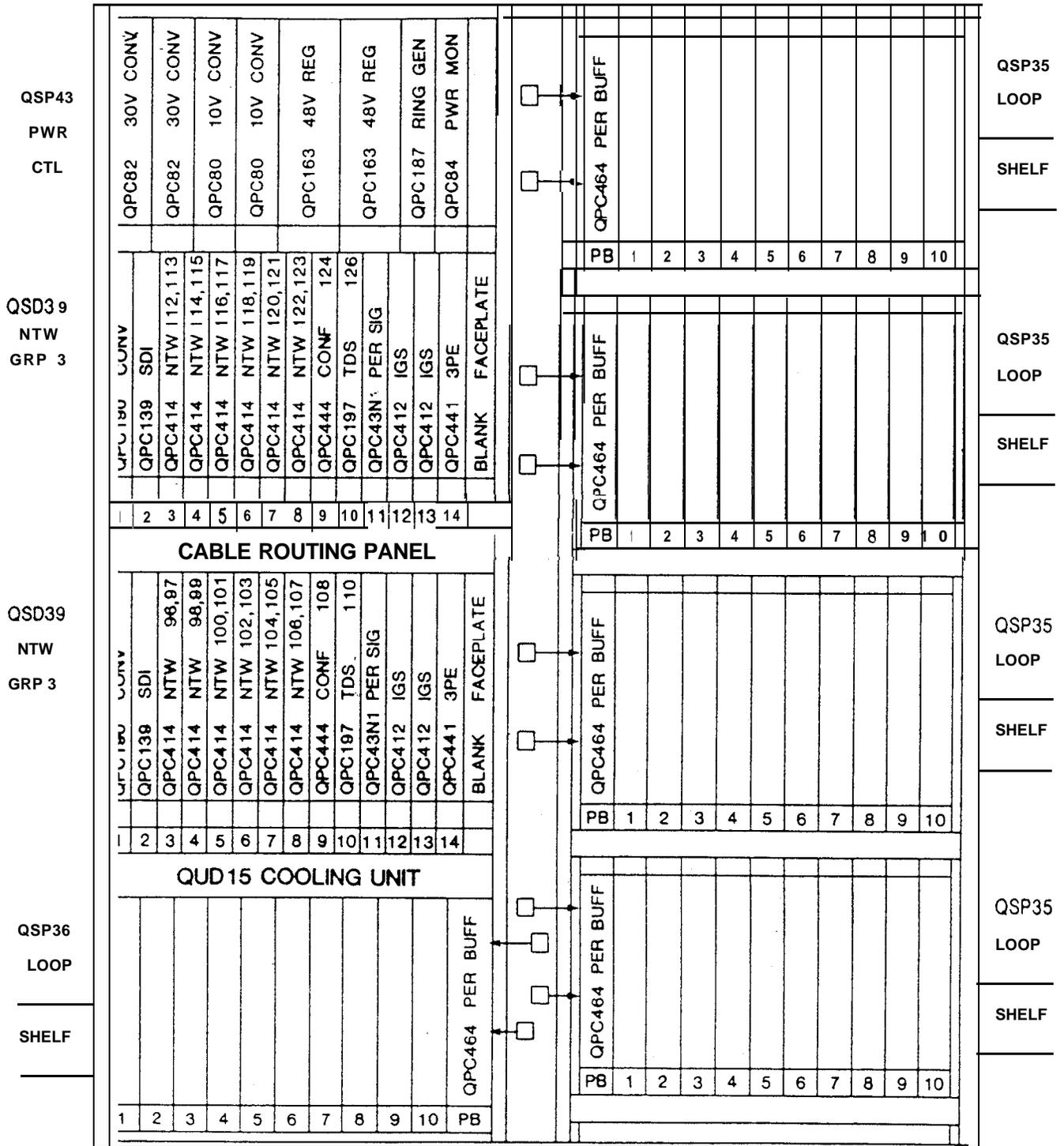
FIGURE 5-28: MERIDIAN SL-1XN QCA108 CABINET • FRONT VIEW
