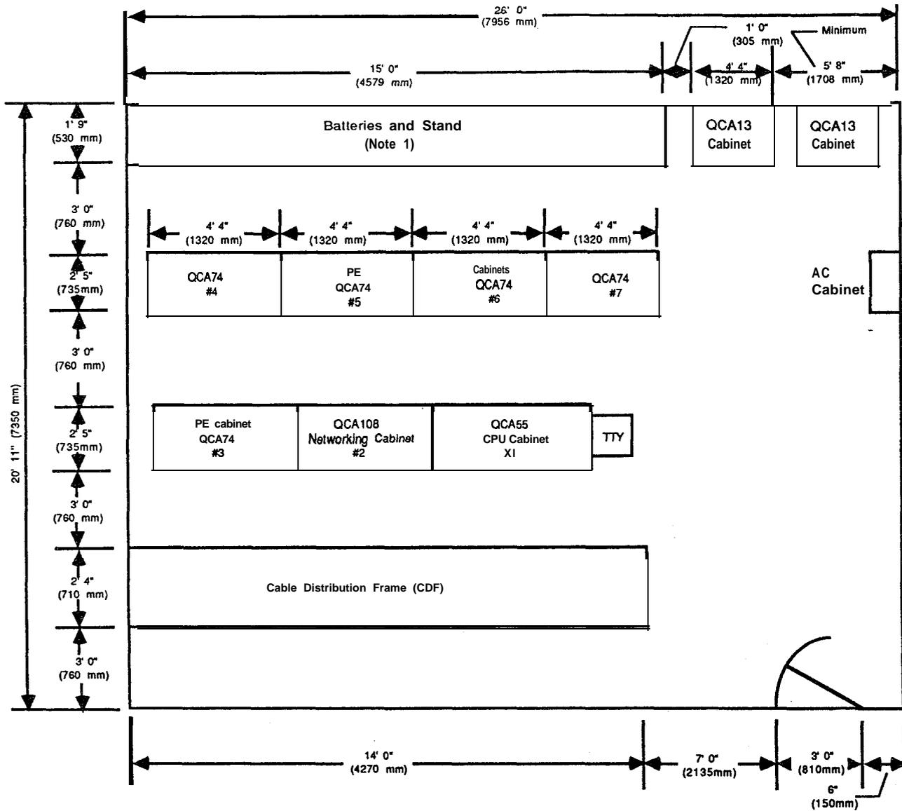
FIGURE 6-2: TYPICAL MERIDIAN SL-1XT FLOOR PLAN
