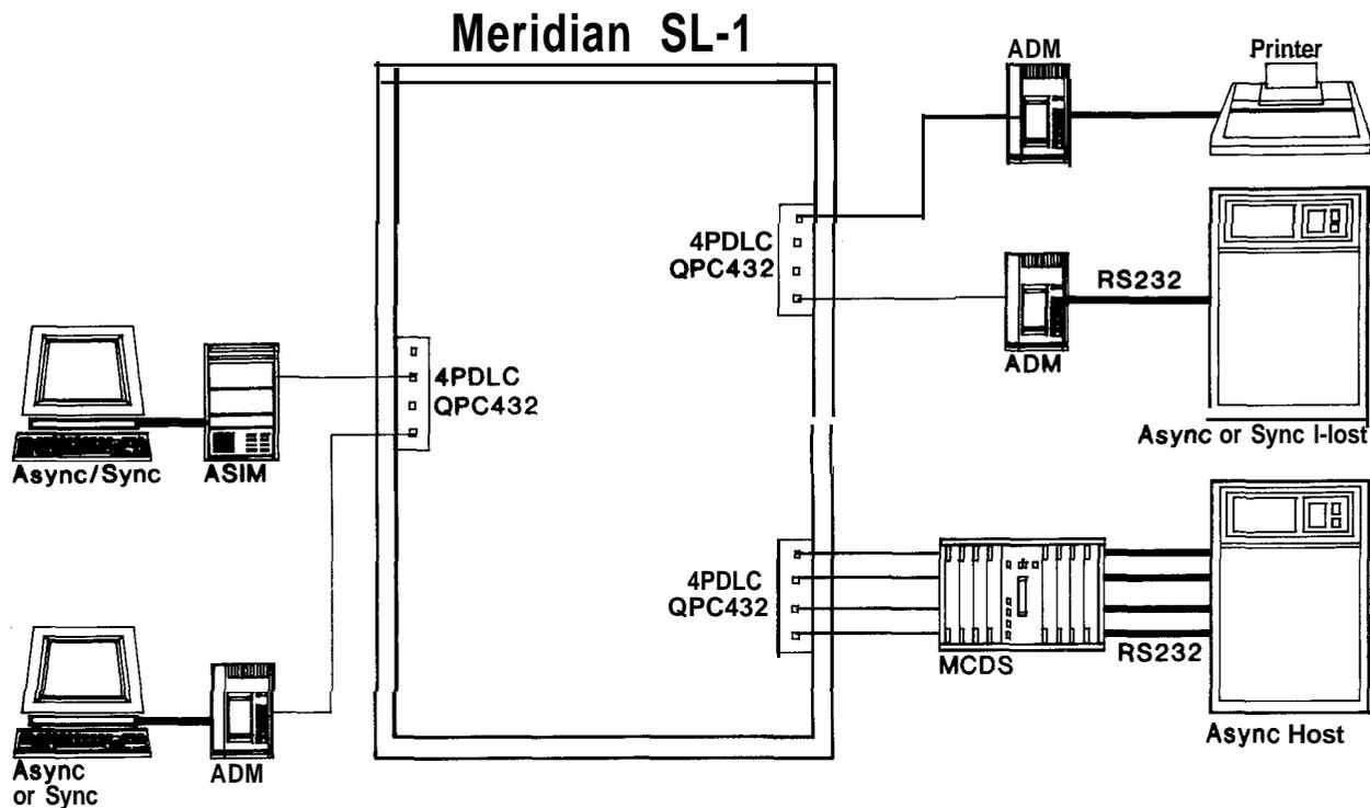
FIGURE 8-32: FOUR PORT DATA LINE CARD
