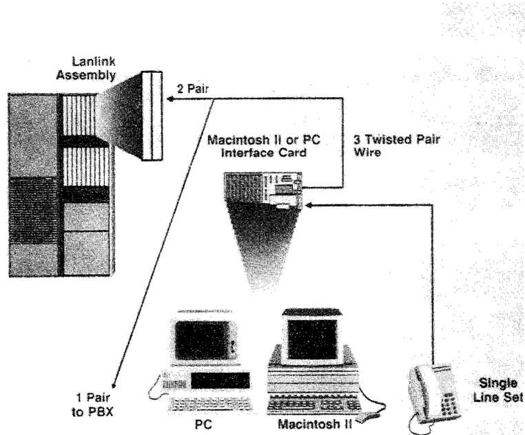
***A LANSTAR PC or Macintosh II Interface Card is installed in each personal computer. A second RJ-11 jack is provided on the card to plug in a telephone. Standard telephone wiring connects the personal computer to the LANLINK Assembly residing in the Meridian LANSTAR packet transport.***
