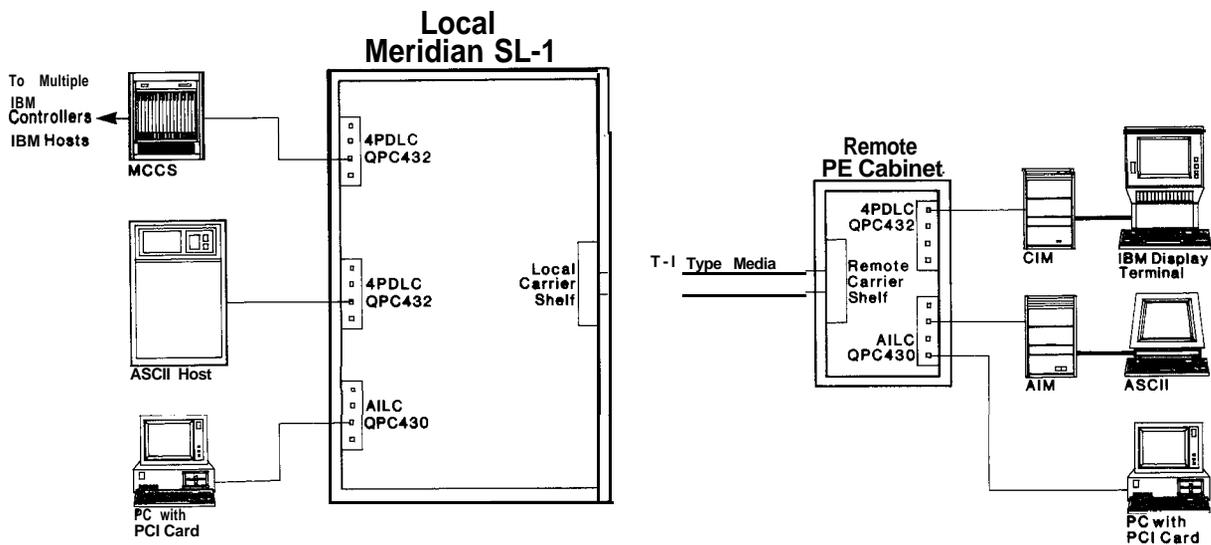
FIGURE 8-26: REMOTE PERIPHERAL EQUIPMENT
