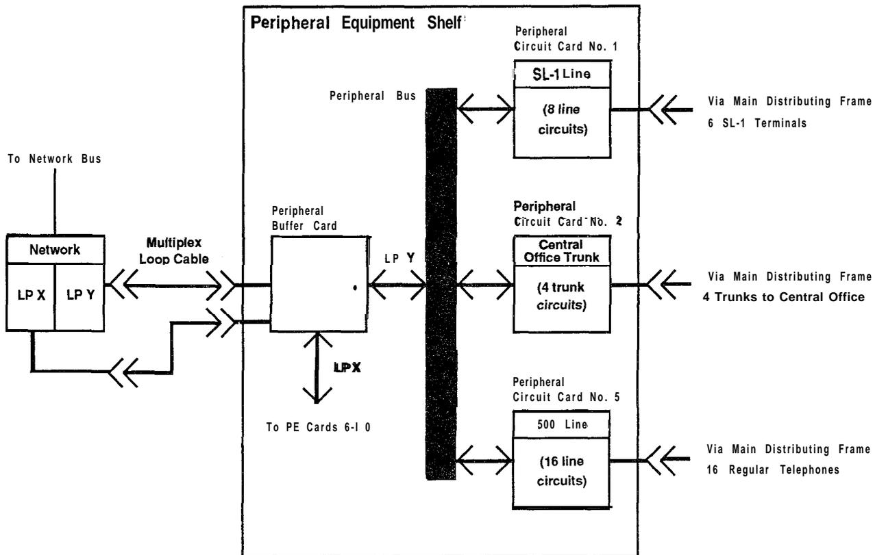
*The functional organization of a PE shelf is illustrated here. A peripheral buffer card drives signals to and receives signals from the peripheral bus on the backpanel of the shelf. The buffer interfaces associated peripheral cards of any mix*
