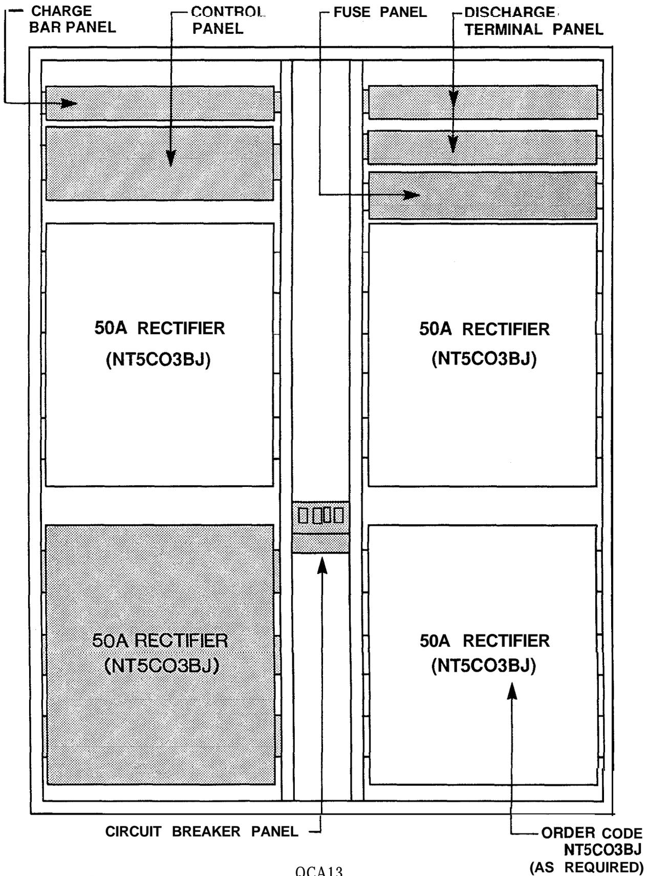
FIGURE 10-20: MERIDIAN SL-1XT MAIN POWER CABINET ASSEMBLY
