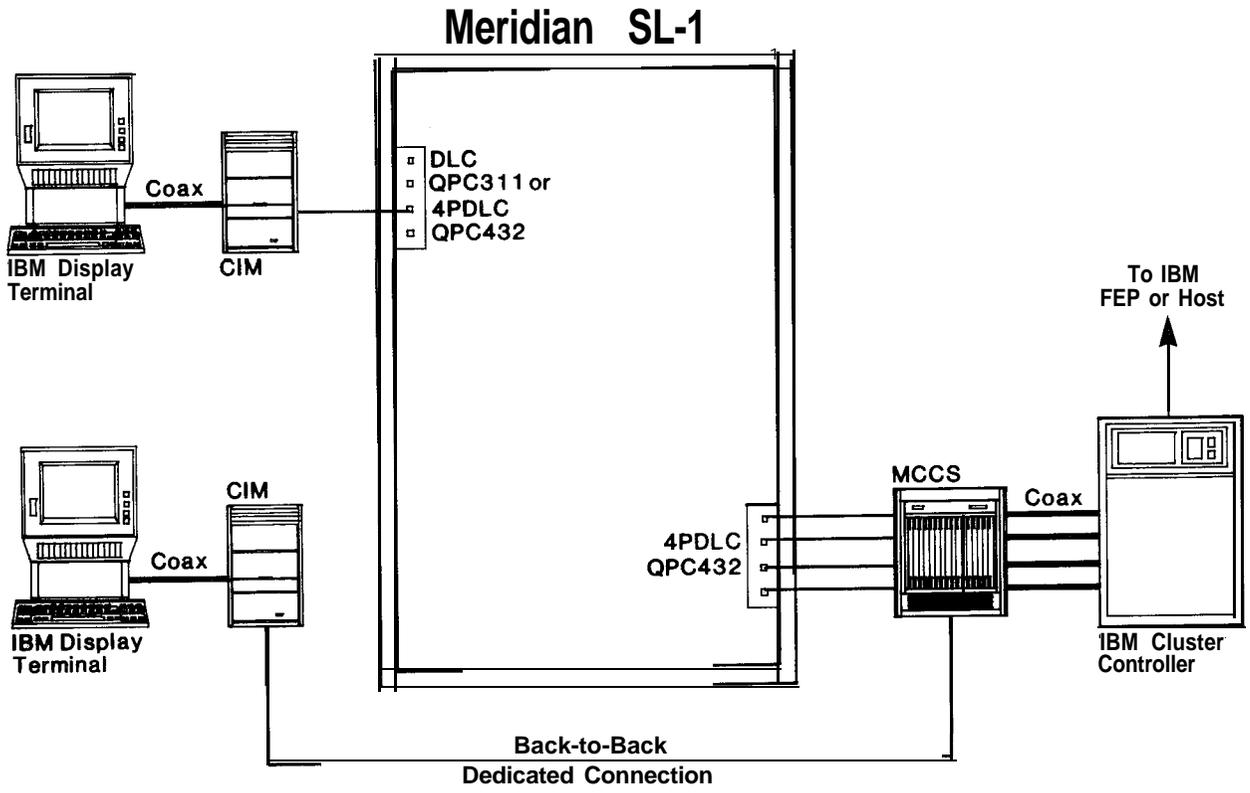
FIGURE 8-23: COAX ELIMINATION AND SWITCHING SYSTEM
