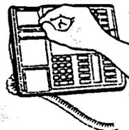
3. Use a screwdriver or similar tool to remove the center knock-out panel in the wall-mounting base.
