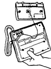
6. Route the line cord through the appropriate cord guide in the bottom of the telephone.
