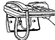
7. Connect the other end of the line cord to the wall jack. Store any spare cord neatly in the base of the telephone and mount the telephone on the base.
