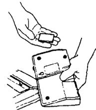
4. Screw the base to the wall (thin end up) so that the wall jack projects through the knock-out.
