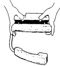
2. Remove the receiver clip from the wall-mounting base. Install the clip in the forward lip of the receiver rest.
