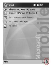
When the **Bluetooth** icon is blue, Bluetooth is active. When the icon is grayed with a red X, Bluetooth is inactive.
