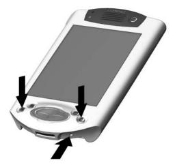
2. Press the **Reset** button on the bottom of the iPAQ Pocket PC with the stylus.
