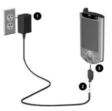
**CAUTION:** Incorrectly inserting the charging adapter plug into the connector on the bottom of the iPAQ Pocket PC can damage the connector pins.
