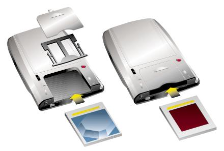
If the card is Type I extended, remove the door from the CompactFlash Type I extended card slot, as shown on the left.
