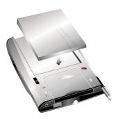
2. Install the backup battery. The CR-2032 coin-cell backup battery is attached to the Quick Start Card. Use the stylus to hold the backup battery lock in the OPEN position, and remove the backup battery tray. Place the backup battery in the tray with the + sign facing up. Slide the tray into its slot until it locks into place.
