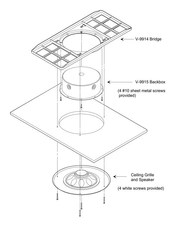
NOTE: The V-9914 must be used in conjunction with the V-9915 when installing the V-1060A, V-1060B, V-1020C or V-1220.
