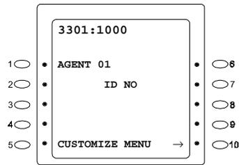
4. Enter 4-digit ID number using the 10-key pad. (The figure on left shows setting of Agent No.01.) To clear ID press **CONF** key.
