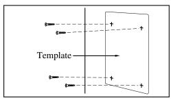
2. Drill holes and drive the anchor plugs (user-supplied) with a hammer, flush to the wall.
