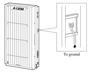
In most of the continental United States, the ground provided by the "Third wire ground" at the commercial power outlet will be satisfactory. However, in a small percentage of cases this ground may be installed incorrectly. Therefore, the following test procedure should be performed.
