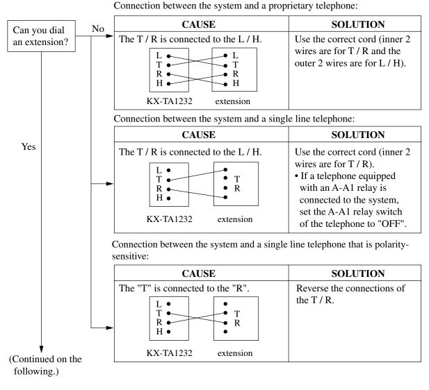
Connection between the system and a proprietary telephone:
