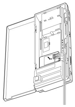
**2.** Loosen the screws on the terminal strip.
