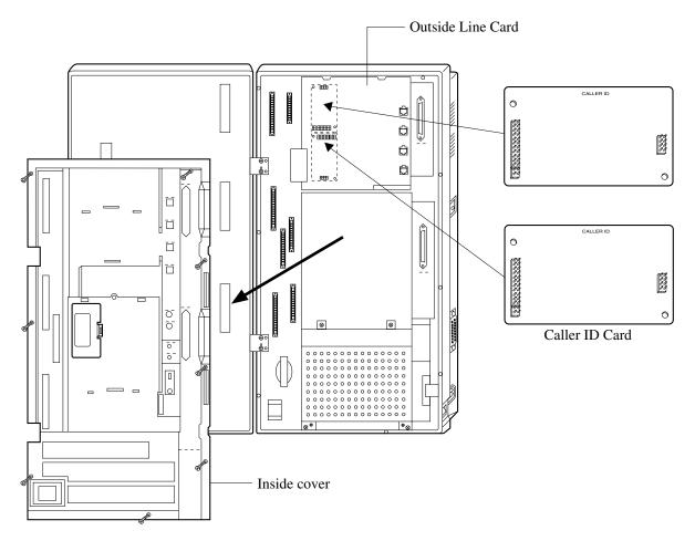
3. Put the inside cover back on the main unit and secure the screws.
