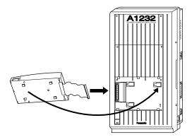
**3.** Hook the cabinet on the main unit and slide the cabinet to the left until it is secured.
