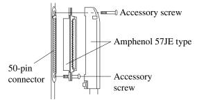
**2.** To attach the Amphenol 57JE type (Plug) to the connector, drive the accessory screw into the upper part.
