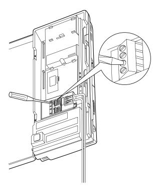
**3.** Insert the wires coming from the door openers into holes and tighten the screws. Pass all the wires through the Holder.
