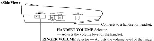
**VOLUME** Control — Adjusts the volume level of the speaker volume.
