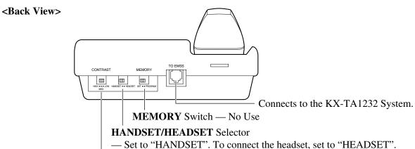
**CONTRAST** Selector — Adjusts the contrast of the Liquid Crystal Display.
