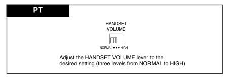
• You may also adjust the handset receiver volume during a conversation using the handset receiver.
