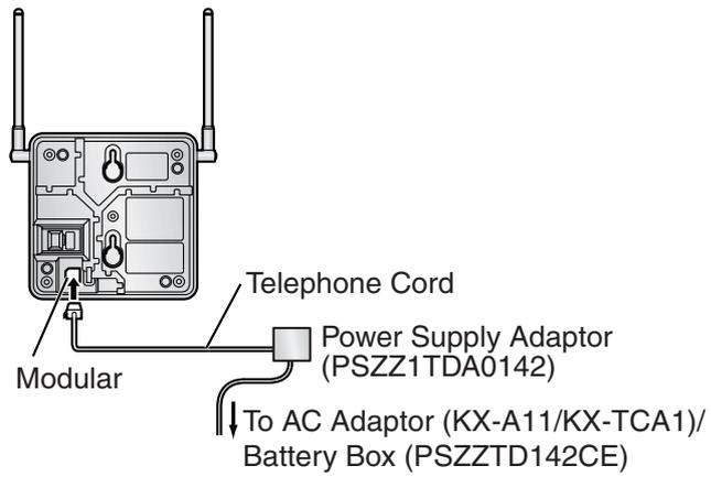
4. Install the CS temporarily for the site survey. Install the CS at least 2 m (6.6 ft) above the floor, keeping the antennas in the upright position.
