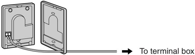
4. Re-attach the 2 halves and re-insert the screw.
