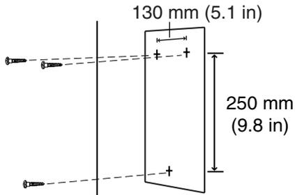
2. Install the screws and washers (included) in the wall.
