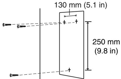
2. Install three anchor plugs (user-supplied) in the wall.
