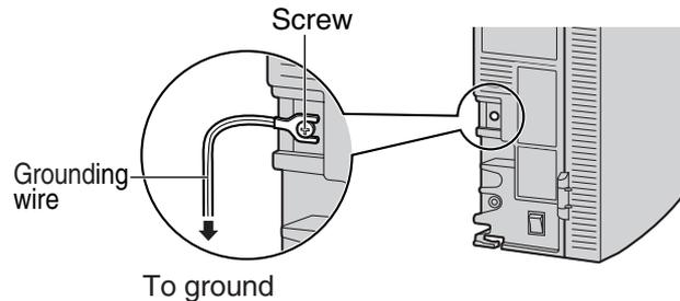
\* For grounding wire, green-and-yellow insulation is required, and the cross-sectional area of the conductor must be more than 0.75 mm<sup>2</sup> or 18 AWG.
