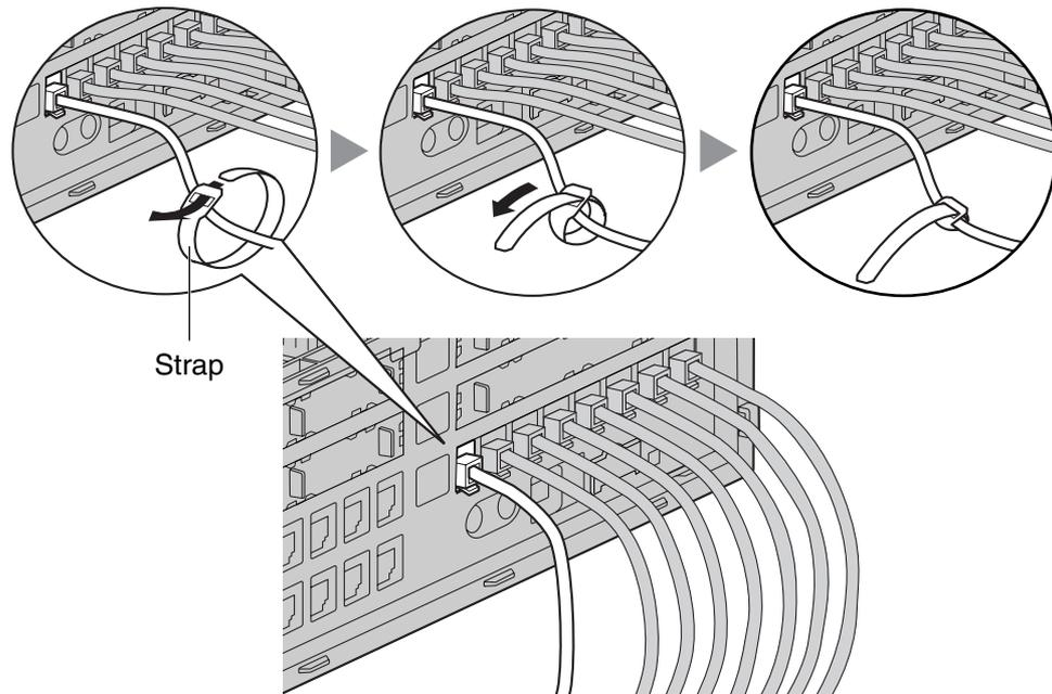
2. Bind all the connected cables together using the strap.
