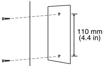
2. Install two anchor plugs (user-supplied) in the wall.
