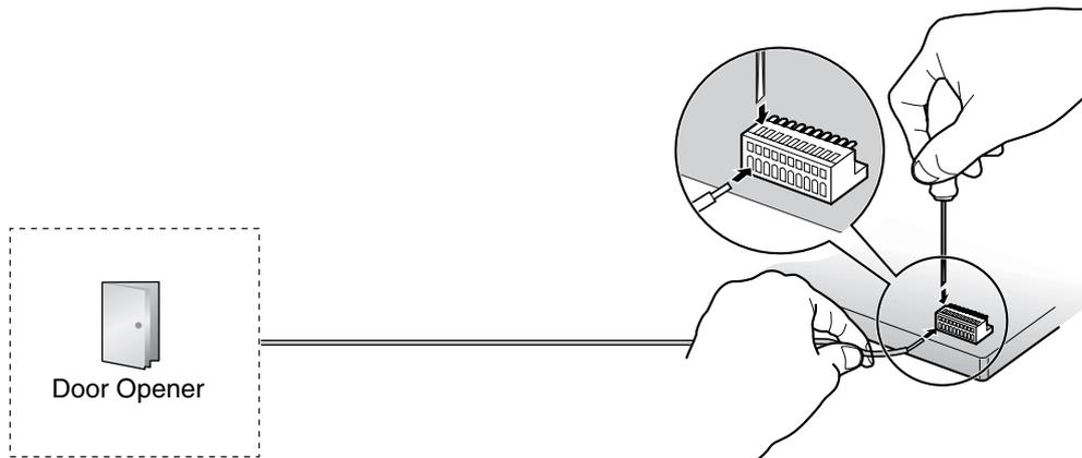
2. Attach the terminal blocks to the connectors of the DPH4 card in the PBX.
