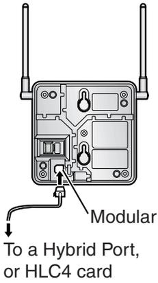
2. Pass the cable through the groove of the CS (in any direction depending on your preference).
