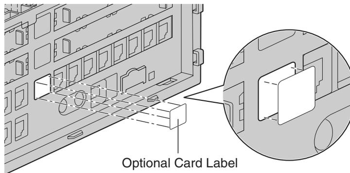
5. Connect a cable to an appropriate port of the card.
