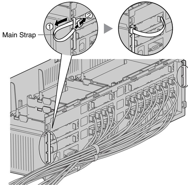
5. Bind all the connected cables together using the main strap, and then close the cable cover. For how to close the cable cover, refer to "2.2.3 Opening/Closing the Covers".
