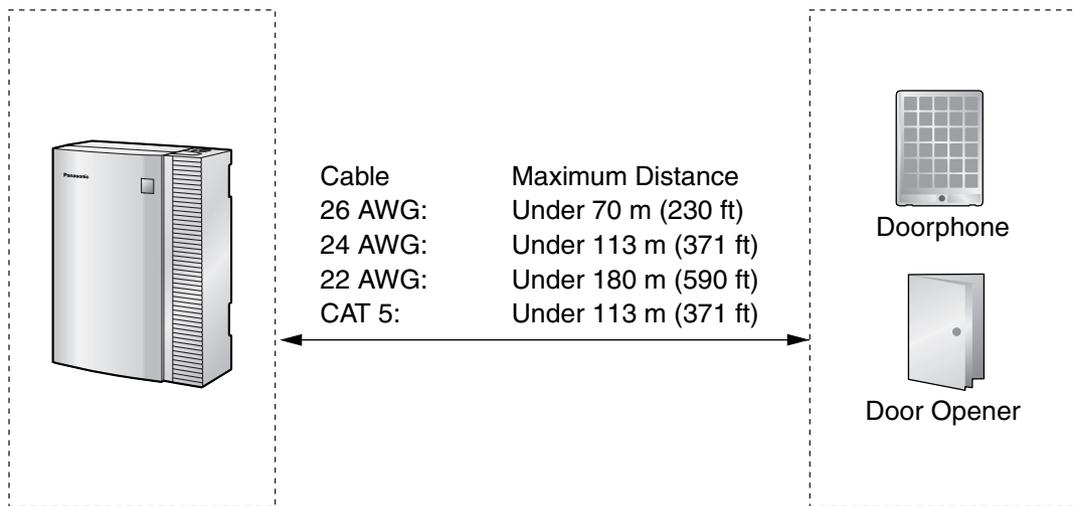
**Current Limit for door opener: 24 V DC/30 V AC, 1 A maximum**
