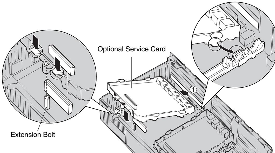
3. Insert the new extension bolt (included with the card) into the hole on the card, and tighten it to secure the card.
