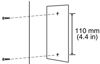
2. Install the screws and washers (included) in the wall.
