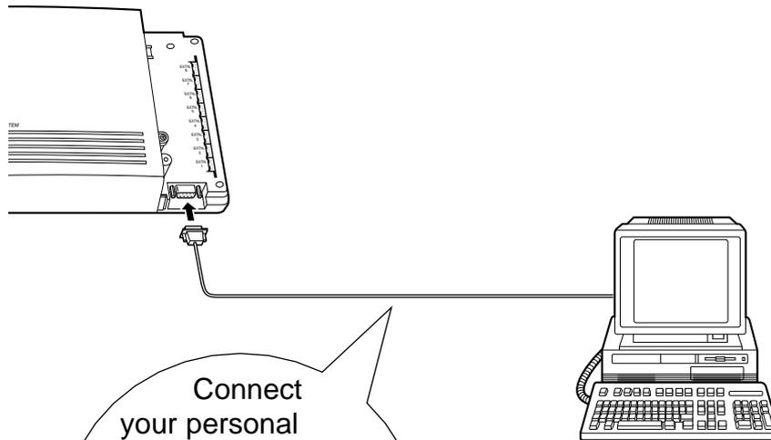
Connect your personal computer to the RS-232C port with the user-supplied serial printer cable. The Cable must be shielded and the maximum length is 2 m.
