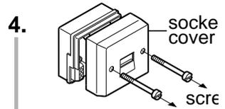
Remove the socket cover with flathead screwdriver.
