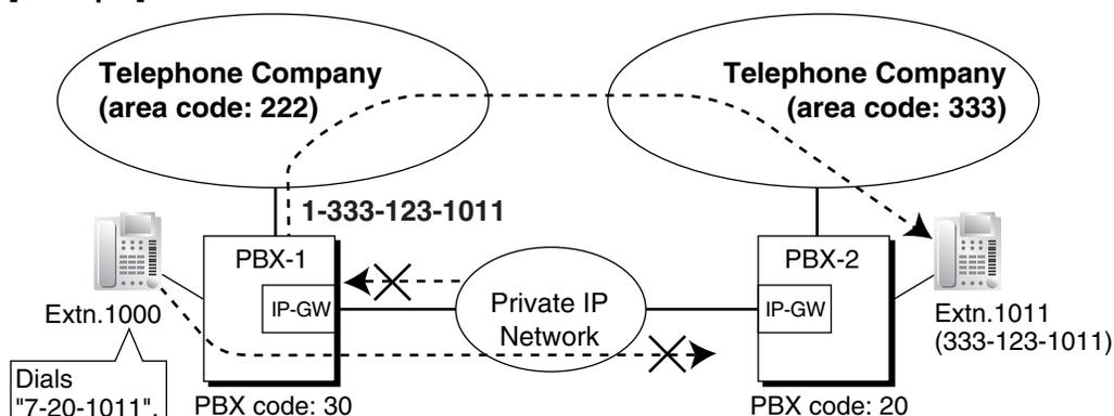
The leading numbers of extensions accessed through the VoIP network are added as entries to the Quick Dialing table, in addition to being registered as Other PBX Extension Numbers, as shown below:
