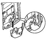
3 Connect the telephone line cord. Mount the unit, then slide down.
