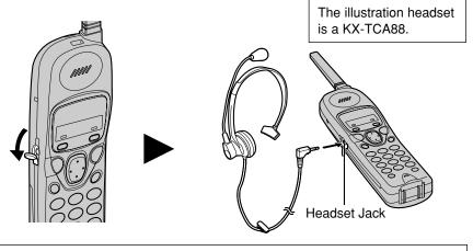
To switch to the speakerphone while using the headset: Press . To return to the headset, press .
