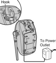
3 Tuck the telephone line cord inside the wall mounting adaptor, then push the adaptor in the direction of the arrows (1) and (2).
