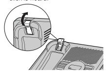
2 Press the tabs in the direction of the arrows (1), then remove the wall mounting adaptor (2).
