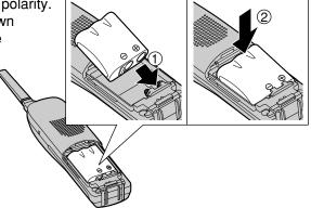
Glose the cover. Make sure you charge the new battery for about 15 hours in order to display the battery strength prompt correctly (p. 14).
